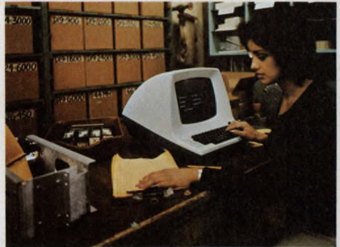
Known as the Dumb Terminal, this 24-line, 80-character CRT terminal is the equivalent of a glass teleprinter. It sells for under $1000 in single quantities.
