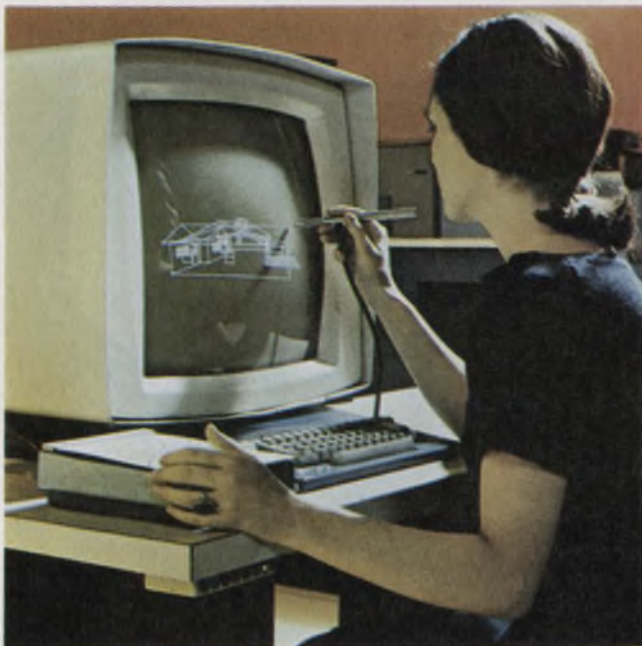
One of the first graphics-display units is this model from IBM. The system is widely used with the company's 360 and 370 large-scale computers.
