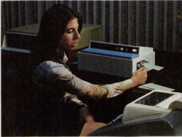
The VER-iCOM-80 from iCOM is a unique instrument that is a combination card reader, printer and computer terminal. The compact peripheral works with \mu Cs.
