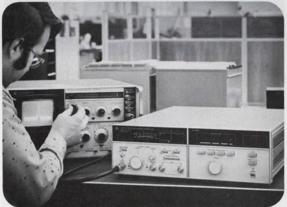
The new HP 8672A Synthesized Signal Generator with wide dynamic range and exceptional stability provides features important to both broadband testing or to highly stable receiver tests.
