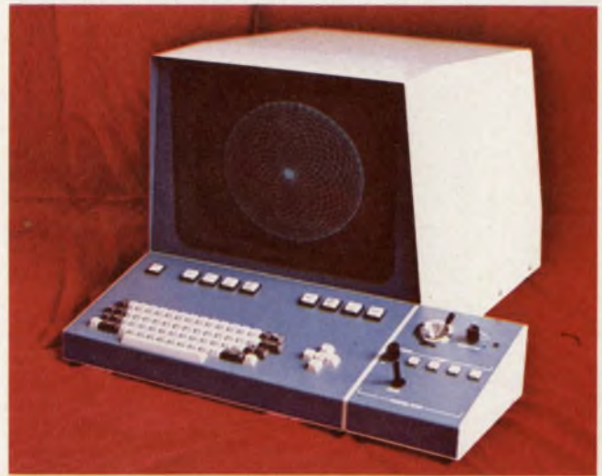
Scan-conversion systems, like this one from Princeton Electronic Products, retain data on a silicon storage tube and use a standard CRT for display.
