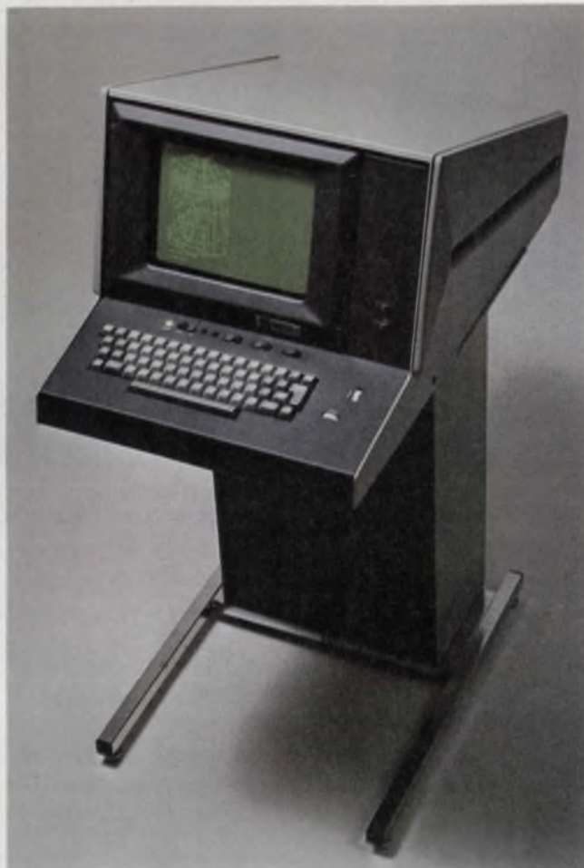
Structural analysis performed on a Tektronix storage-tube terminal provides geometric previews of a section of a diesel-engine piston.
