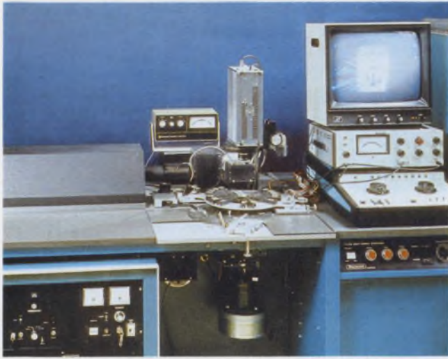
Laser trimmer sets FSK frequencies precisely for Cermetek's hybrid modem modules. The unit trims the frequency determining resistors for the 300-baud set.
