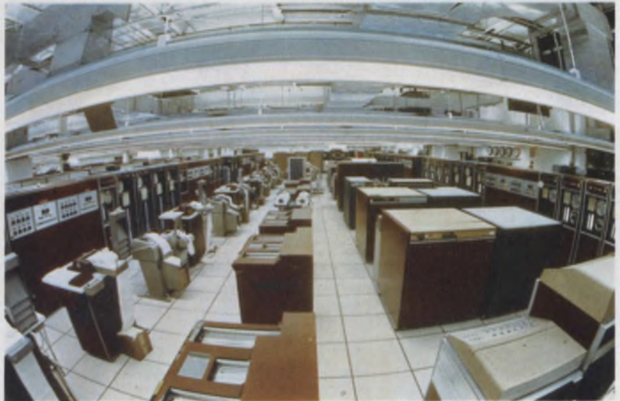
The General Electric Supercenter near Cleveland is the heart of the world's largest time-sharing computer network. It contains 15 large scale computer mainframes which comprise the bulk of the Mark III system.
