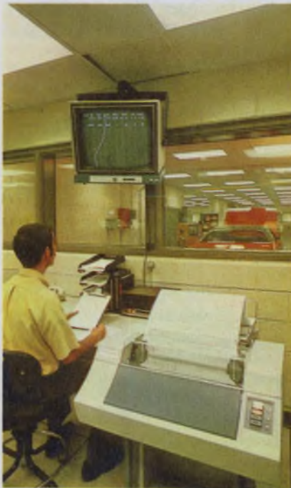
Centronics 101 dot-matrix printer records data at Chrysler's vehicle-emission center in Detroit. The 101 prints at 165 cps.
