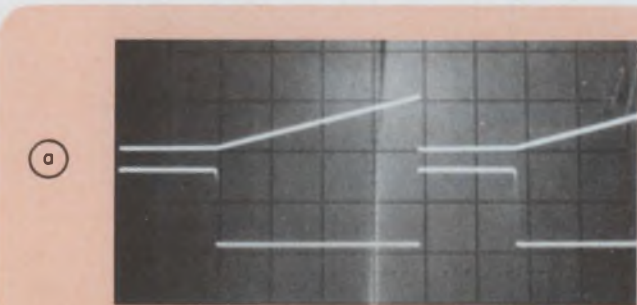
3. The sweep generator covers easily a wide range of speeds; traces range from 0.5 ms to 0.5 \mu s per div.
