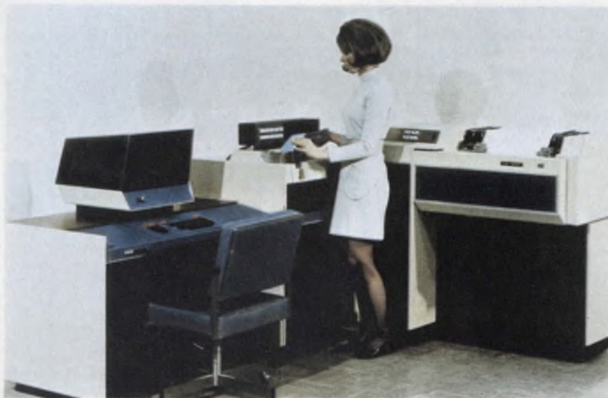
Remote batch system from Control Data can be used to support a number of engineering users by providing high speed data entry and printing capability without tying up individual terminals.
