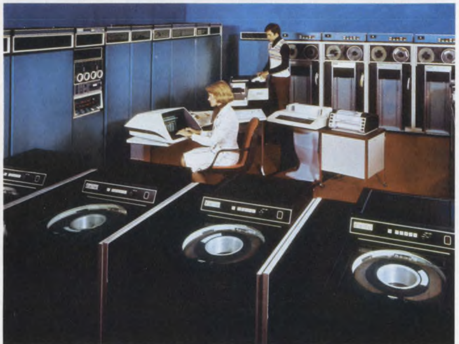
The KL-10 central processor for the DECsystem 1080, a large-scale interactive computer, uses ECL logic and a cache memory for operation at very high speed. Typical of an architectural trend, the KL-10 features a PDP-11/40 as a control/diagnostic console that troubleshoots the entire system.
