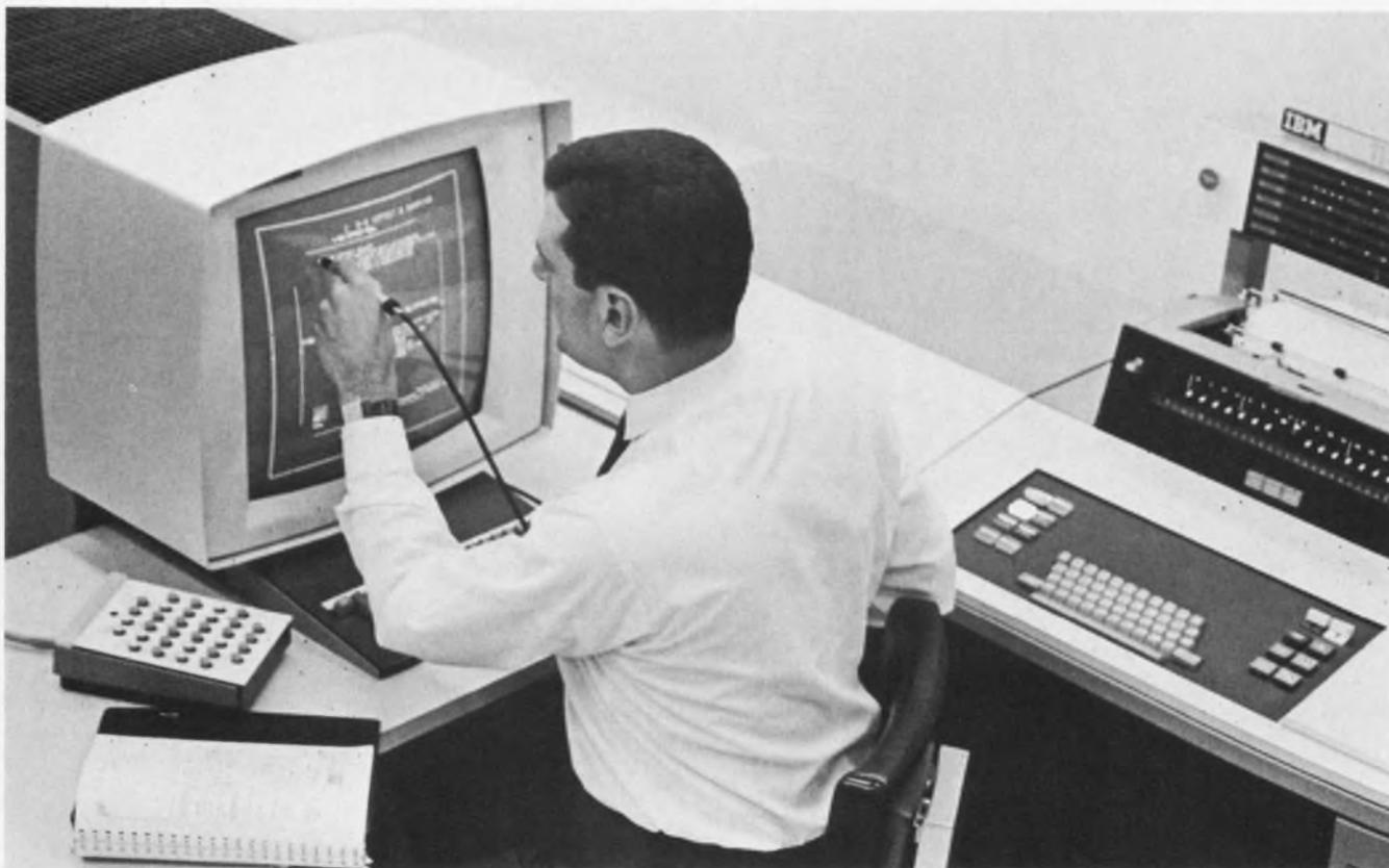
An operator is using the IBM 1150/2250 Stand Alone/Remote System. A program correction is being made by
