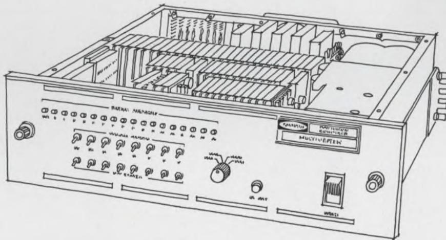
Faster throughput is just one of the benefits offered by the MULTIVERTER III, newest version of our widely-used "analog front end in a box." Multiplexer capacity can be up to 128 channels, the sample-and-hold amplifier has a 2 microsecond settling time and 50 nanosecond aperture, and the converter is our new 15-bit, 0.01% ADC 100.
