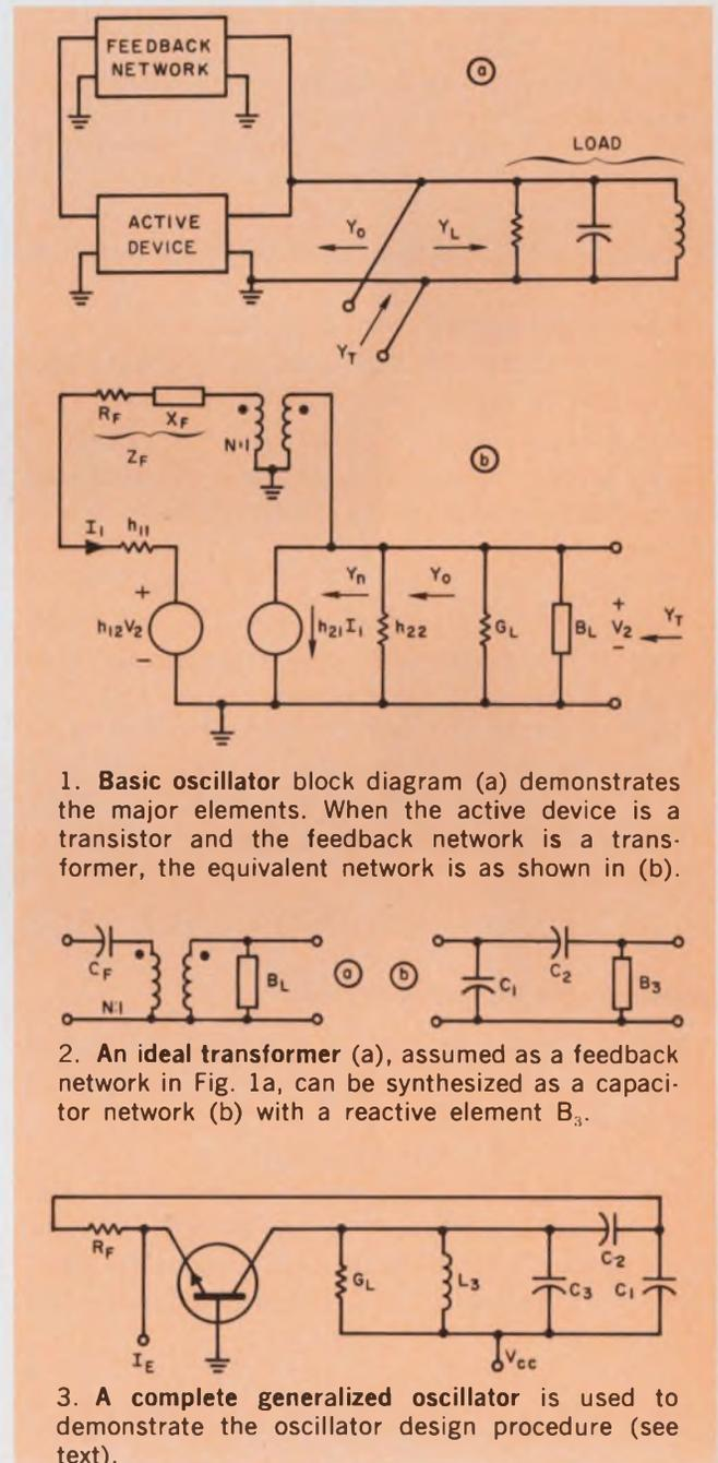
1. Basic oscillator block diagram (a) demonstrates the major elements. When the active device is a transistor and the feedback network is a transformer, the equivalent network is as shown in (b).
