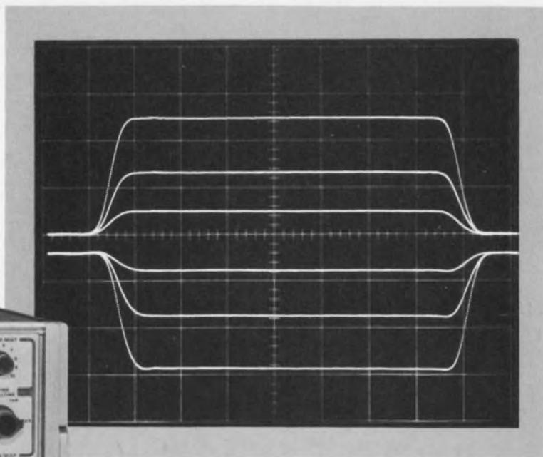
Multiple exposure showing typical waveform aberrations for positive and negative polarities at various amplitude settings. Notice the constant risetime and falltime with amplitude changes. 20 ns/cm sweep time and 4 V/cm deflection factor.
