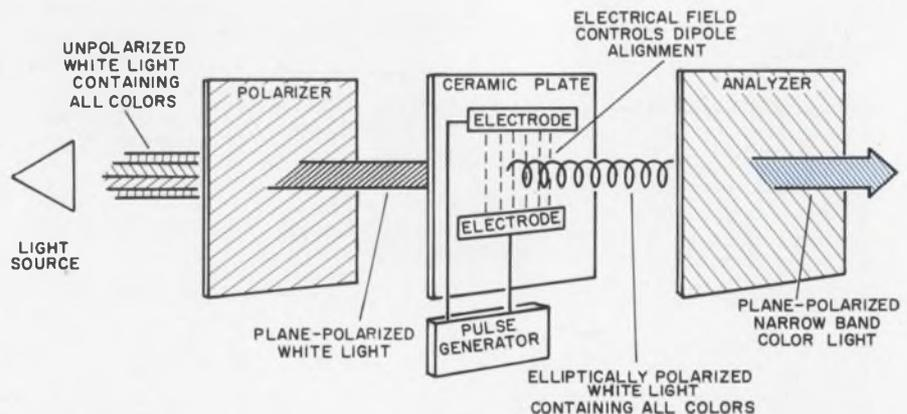
wires extending from the larger electrodes. Illustration shows how polarized white light is converted into plane-polarized color light.
