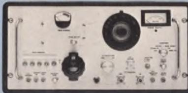
Outputs to 40 watts — leveled swept output up to 8 watts — frequency coverage from 20 to 1000 MHz — sweep widths to 15%—sweep or CW modes — birdy frequency markers.
