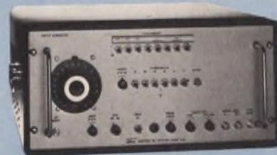
Four single chassis models — 20 kHz to 900 MHz — continuously variable sweep widths—birdy frequency marking — high stability, low VSWR — 50 or 75 ohm versions.
