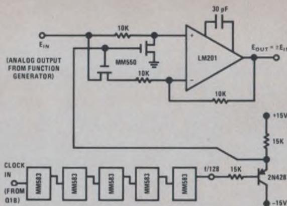
FIGURE 4. Analog Inverter Reverses Polarity of Periodic Functions.
