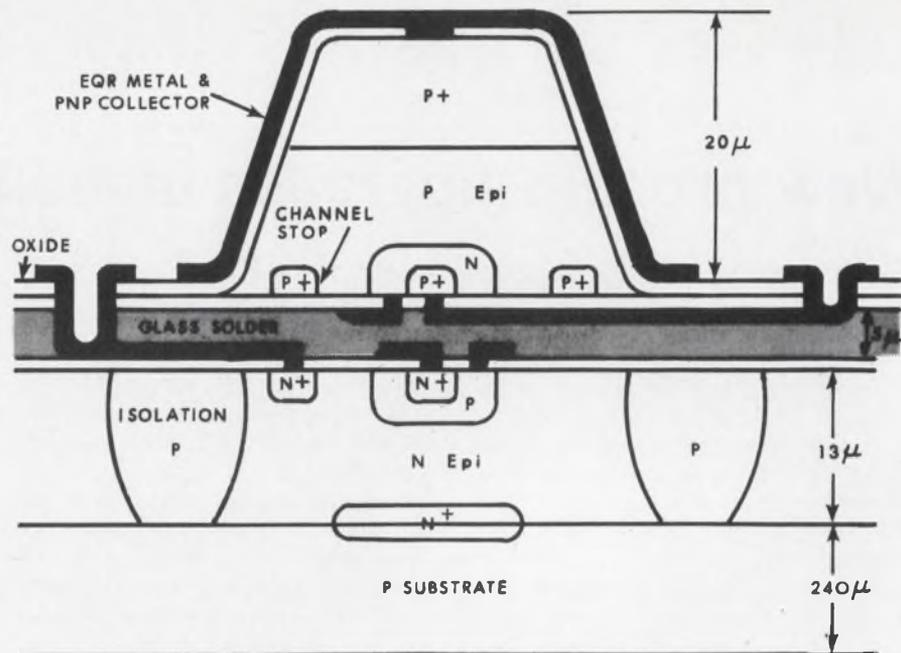
2. The pnp wafer is back-lapped to a thickness of about 20 microns, and individual devices are mesa-isolated by standard masking and etching techniques. Interconnection metalization is applied by standard processes through the oxide layer and solder, to make contact to the original wafer metalization.
