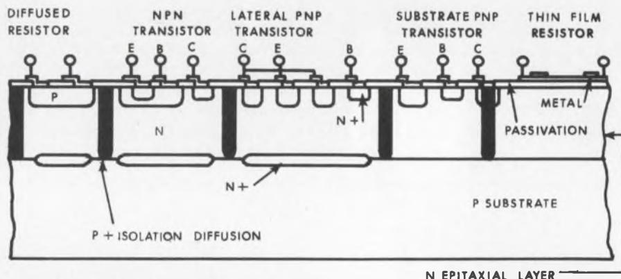
3. Other methods for making pnp transistors have serious disadvantages. Lateral pnps have low gain and are subject to contamination, and substrate pnps tend to be slow because the base region is very wide.
