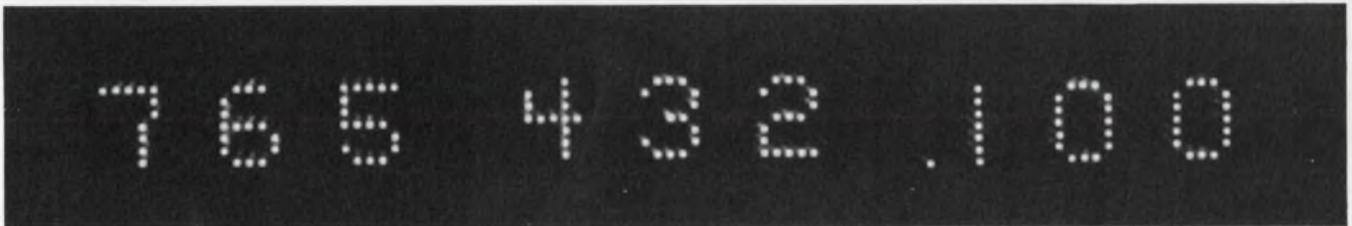
**Solid-state indicators** display an array of bright red dots in numeral form. The thin,
