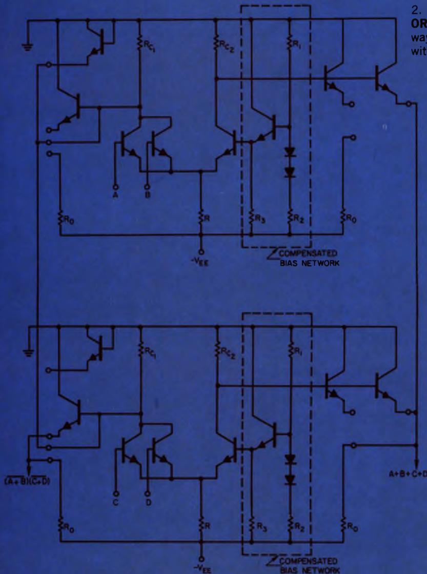
2. The ECL configuration allows WIRED-OR and WIRED-AND connections. In this way extra logic gating can be performed without adding delay.
