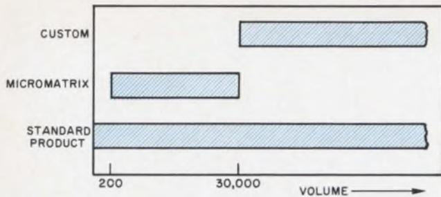
3. **Medium volume complex circuits** are often not standard products and are not required in sufficient volume to justify custom design. A special approach, which allows a limited amount of customization, is required for this market area.
