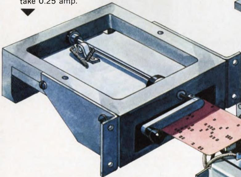
**Solenoid badge reader.** Model 360. Reads 15-, 20- or 22-column badge — up to 264 switches. Operates similar to time clock. Models for 115 VAC and 28 VDC. Design life: one-half million cycles.
