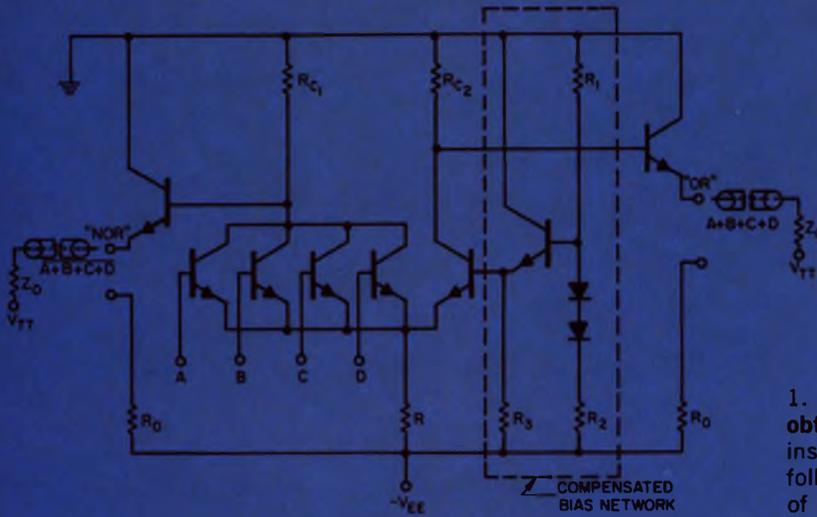
1. Nonsaturated logic circuits are used to obtain high speeds. This ECL gate, for instance, has signal paths through emitter followers and grounded-base stages, both of which are inherently fast.
