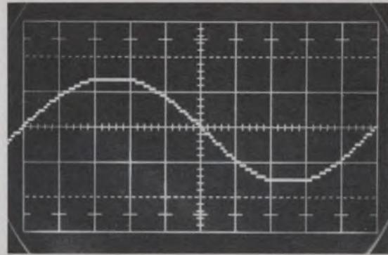
FIGURE 1. Typical Scope Trace Produced by MOS Memory.
