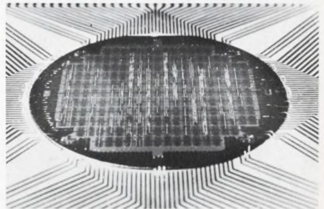
1. A discretionary-wired LSI wafer is an array of logic circuits that are connected after testing to form the desired complex logic function. The interconnection pattern is different for each wafer, and uses only the good circuits.
