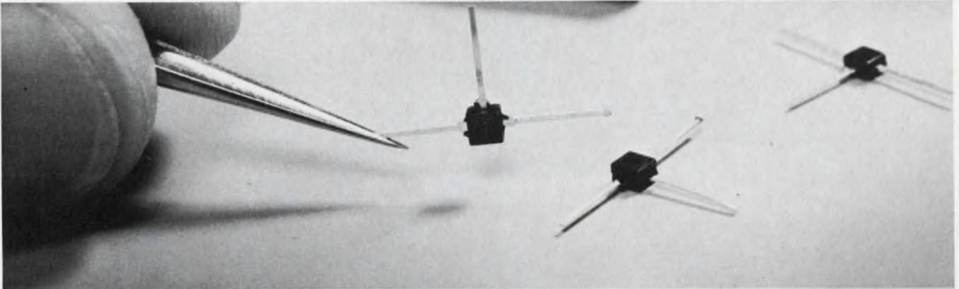
**Miniature silicon transistors** feature a plastic spider-type package that occupies only 18%
