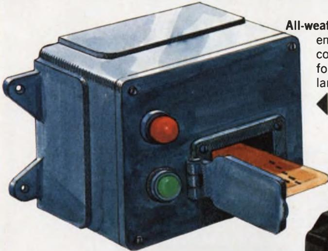
**All-weather reader.** Designed for outdoor or industrial environments. Suitable for air purge system. Bifurcated contacts — up to 264 cross points. Credit card format up to 12 x 22, matrix or individual. Indicator lamps and card release switch available.
