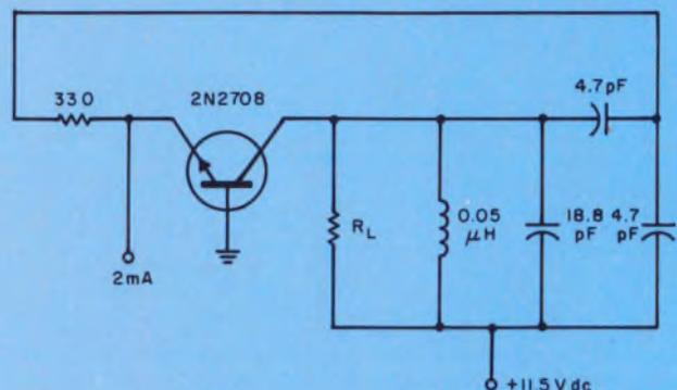
5. This 150 MHz oscillator was designed, step-by-step, to illustrate the proposed design procedure. The 330-ohm emitter resistor is large enough to swamp changes in  $h_{ib}$  without sacrificing drive capability.
