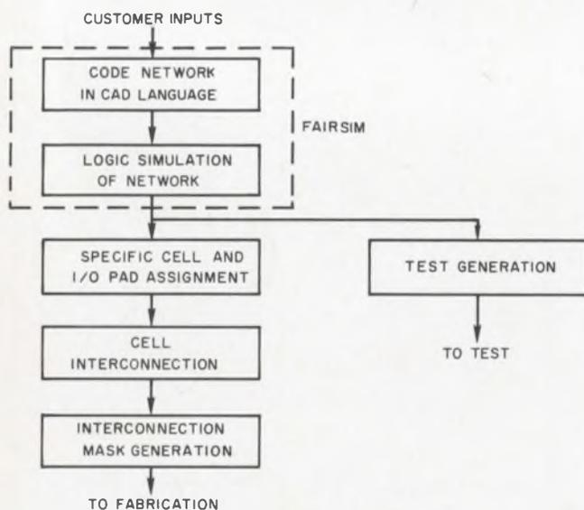
2. In the Fairchild computer-aided design program the customers' logic equations or diagrams are first converted to a CAD compatible format, then simulated to verify the basic design and the network coding. The arrangement of cells in the array is made to simplify the cell interconnection, and the required masks are computer-generated. An optimum sequence of tests is then produced to fully test the custom circuit.
