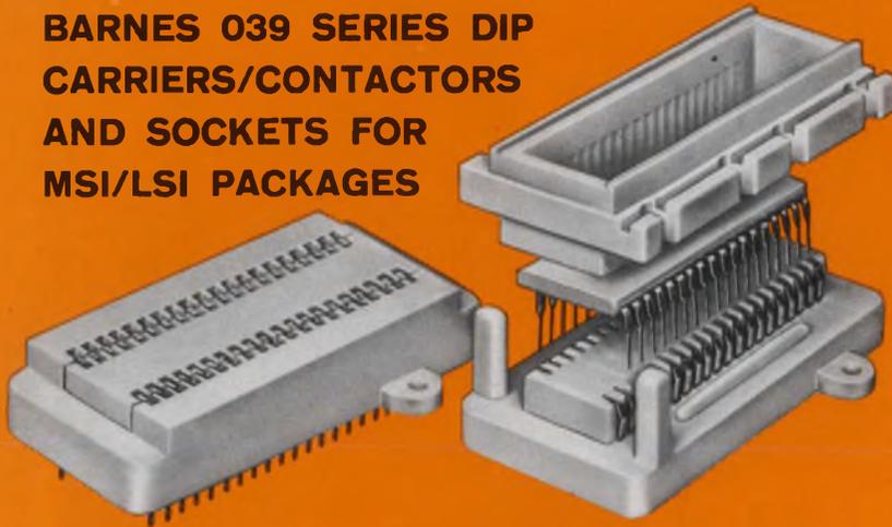
Here are the Big Ones from Barnes! Use them with DIP MSI/LSI packages up to 40 leads, lead spacing of 0.100" and row spacing of 0.500" or 0.600". They eliminate lead deformation in handling, test and shipping, assure reliable electrical contact with positive retention. Carriers and contactors insure correct device polarization. Wiping type contacts in sockets prevent distorting DIP lead taper. Write for the big story.
