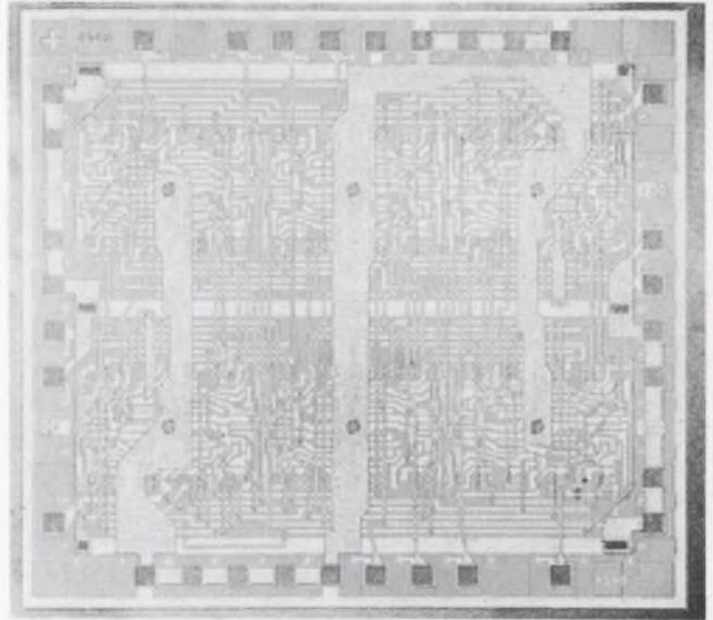
A four-bit carry-look-ahead arithmetic unit, implemented with the 4700 array, performs any of eight parallel functions on two 4-bit operands. The functions include ADD, SUBTRACT,  $A \cdot B$ ,  $A \cdot \bar{B}$ ,  $A + B$ ,  $A + \bar{B}$ ,  $A \oplus B$ , and  $A \ominus B$ . In the subtract mode, the circuit can function as a 4-bit comparator, providing  $A < B$ ,  $A = B$ , or  $A > B$ .
