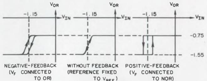
2. Transfer characteristics show the effect of both positive and negative delayed feedback on the ECL circuit.
