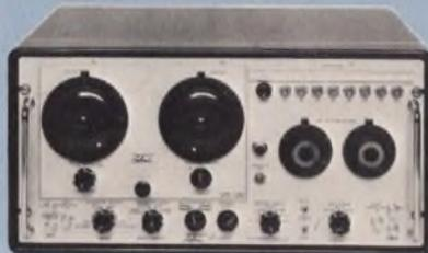
Has 21 plug-in oscillators available — quick adaptability to sweep or signal generating applications — covers 20 Hz to 3 GHz — broad selection of marker types — variable sweep rate — CW operation.
