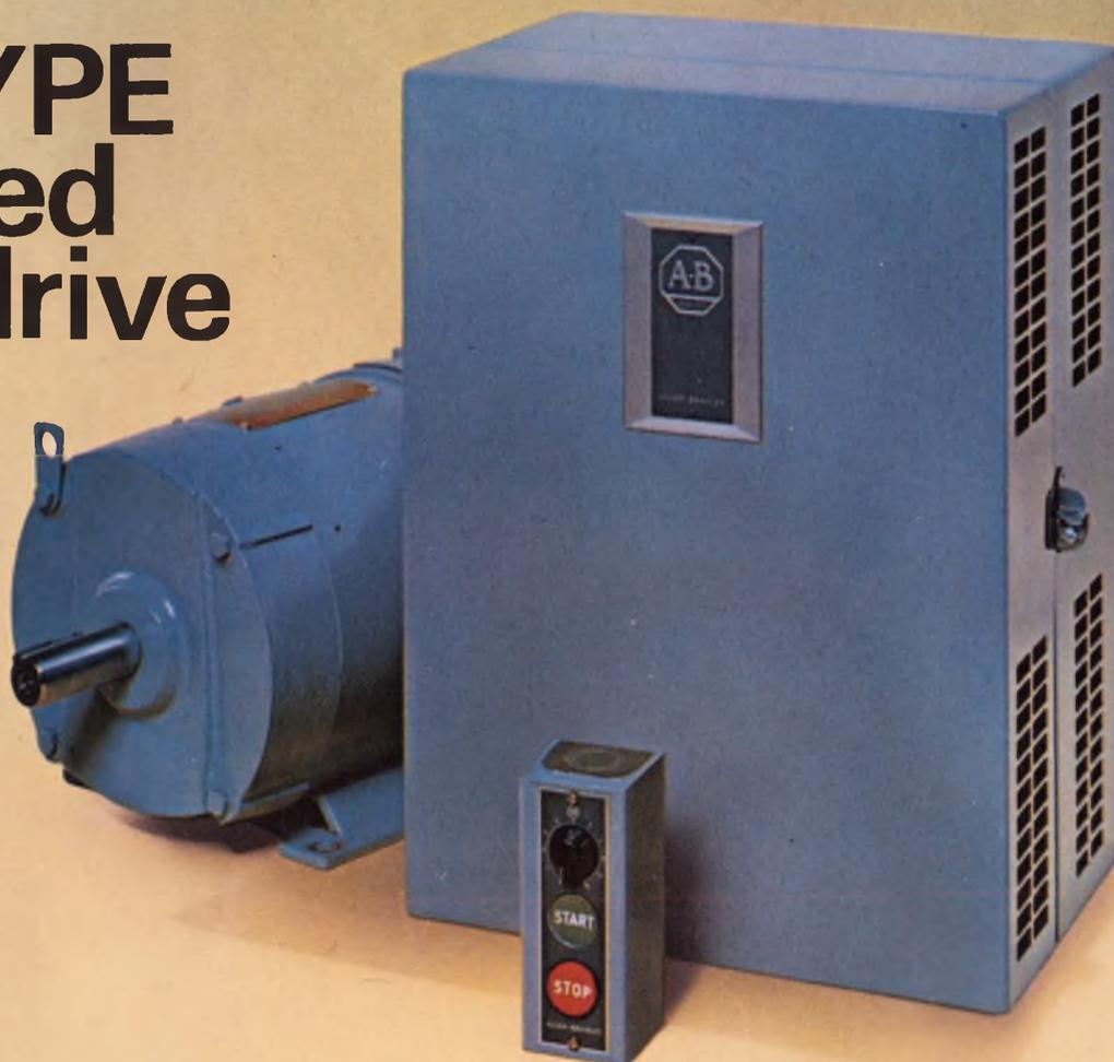
This newest Allen-Bradley regulated speed drive combines a NEMA re-rated integral horsepower motor, an easy-to-wire operator's control station, and a rugged controller matched to provide superior performance. Built to NEMA industrial standards, all three provide traditional high quality for trouble-free service. The SCRs for full wave conversion of the single phase supply are conservatively rated and amply protected. And there's a horsepower rated contactor.
