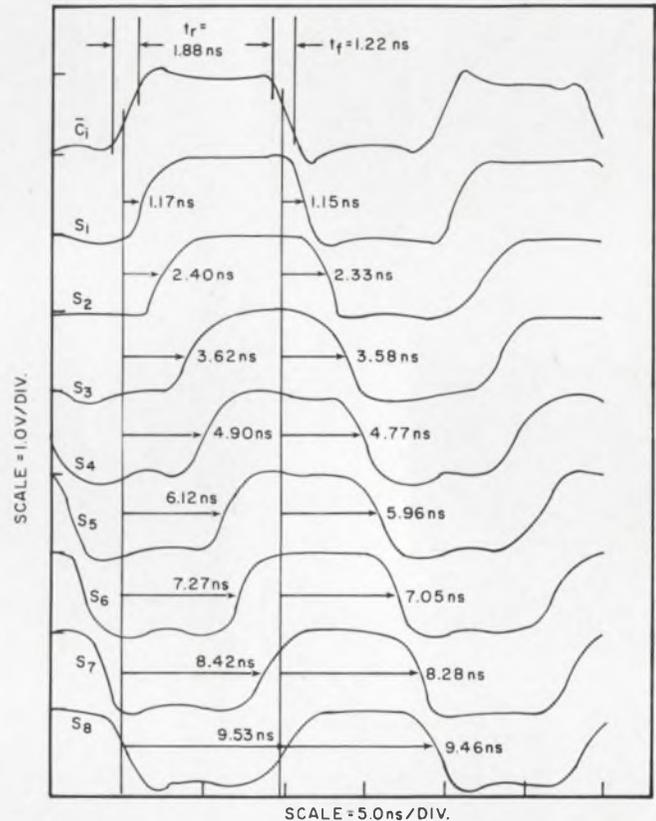
6. The total delay is 10 ns, from CARRY-IN to SUM-OUT, in this 8-bit, ripple-carry adder. This is an improvement of 4:1 over previous standard ECL adders.
