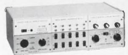
The ADD permits investigation and design of various analog and digital circuits and instruments, by plugging-in circuit cards to its power, binary and timing modules. Connections are made with ordinary wire and component leads.
