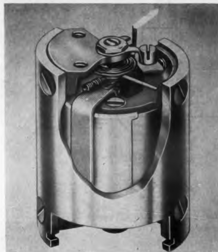
Fig. 1. Providing a 50 \mu amp sensitivity for 180 deg deflection, the assembled meter measures no more than one inch in diameter.
