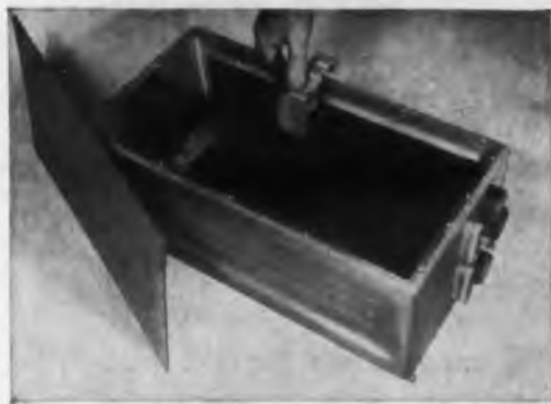
Precision control of groove depth and spacing assures ease of servicing and interchangeability of circuit shells.
