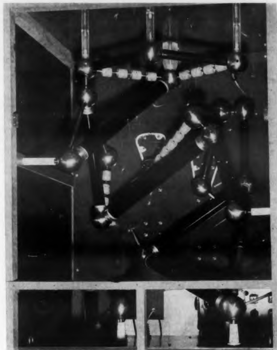
Spark gap circuitry uses 30 in. ribbon-type resistors and anti corona spheres that are 5 in. diam. Three dimensional configuration enables critical spacings to be maintained in a minimum cabinet volume.
