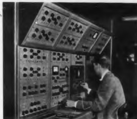
MODEL T88 COMPLEX MOTION CONSOLE equips system for duplicating "noise" or random motion. Uniquely, it contains peak notch equalizer . . . which is an analog computer for giving exact inverse of the resonant response from specimen on the exciter.
