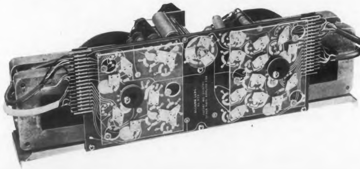
Fig. 2. Demonstration model of a HEP switch used in an octave band filter assembly. Contact board is rotated in a cycloidal motion so that each of the spring loaded contacts describes a perfect circle around its associated circuit. All circuitry is printed on board, capacitors and inductors mounted behind. Contact plate is plexiglas. Note variety of switch shapes on board.
