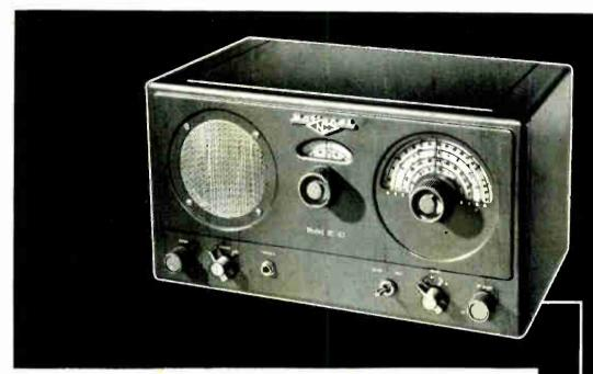
The NC-33 is a real communications receiver covering all frequencies from 500 kc. to 35 Mc. It comes complete with spreaker and AC/DC power supply in an attractive light-weight metal cabinet — carefully produced from components of good quality. It is simple to install and a pleasure to operate. This economical superheterodyne will serve well and reliably. The NC-33 is the perfect choice for your living room, playroom or den.
