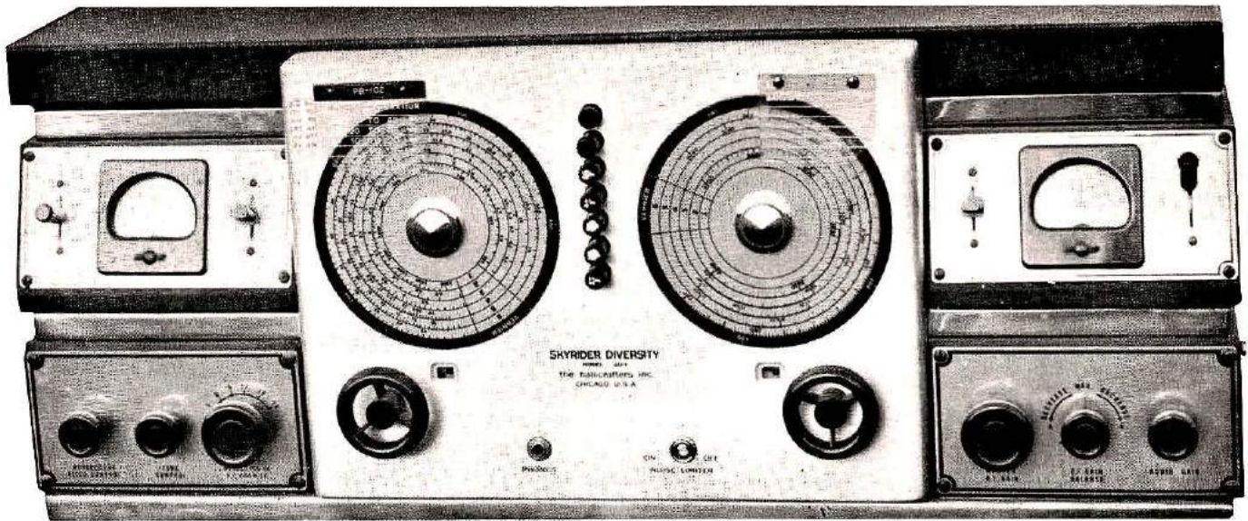
Rare Hallicrafters Skyrider Diversity receiver, which was marketed in the middle of the depression with a price tag of $425 — about six months pay for those who were employed. Only about a dozen of these sets were made. The receiver is about 3 feet (1 meter) long. In spite of its impressive size two additional chassis were used which were installed on either side of the receiver (photo by K4KJ).
