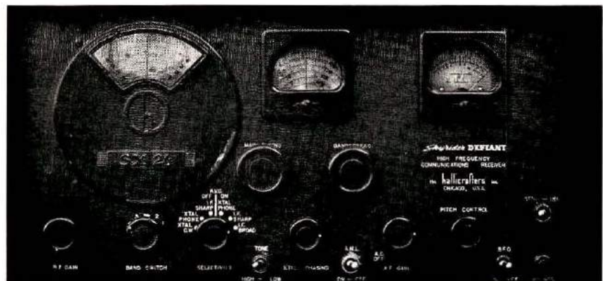
Hallicrafters Sky Rider Defiant was also known as the SX-24. It had one rf stage, two i-f stages, a crystal filter, S-meter, and sold for $69.50 (plus external speaker). One of the features of the receiver was its Frequency Meter Tuning system — when the main tuning dial was set to an appropriate index, the bandspread dial was accurately calibrated and could be used as a frequency meter. K4KJ claims that the one he owned was "dead accurate" (photo by K4KJ).
