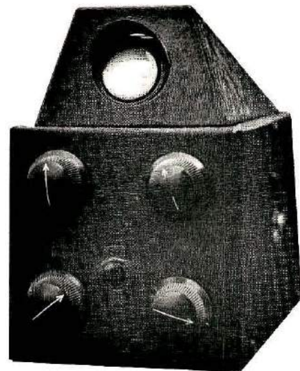
National 1-inch oscilloscope from the late 1930s. After about 1936 all amateurs were expected to know their modulation percentage. The National CRO used a 913 cathode-ray tube; a trapezoidal pattern was normally used because no linear sweep was provided (photo by K4KJ).
