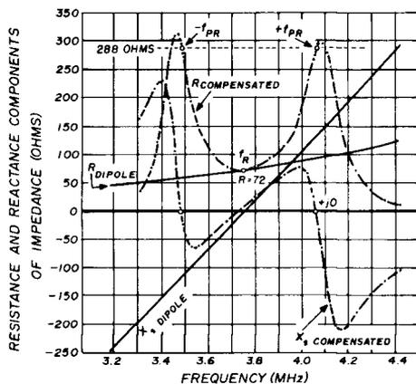
fig. 6. Resistance and reactance components of compensated and uncompensated half-wavelength antennas. Reactance is cancelled at the upper and lower parallel-resonant frequencies  $+f_{pr}$  and  $-f_{pr}$  leaving a resistive component of 288 ohms.
