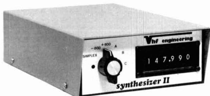
The Synthesizer II is a two meter frequency synthesizer. Frequency is adjustable in 5 KHz steps from 140.00 MHz to 149.995 MHz with its digital readout thumb wheel switching. Transmit offsets are digitally programmed on a diode matrix, and can range from 10 KHz to 10 MHz. No additional components are necessary!
