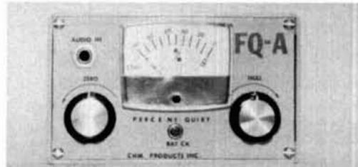
FINELY, A SYSTEM TO MEASURE THE PERCENT OF QUIETING IN FM RECEPTION. ACCURATE AND CONSISTENT PERCENT QUIETING REPORTS PLUS FINE TUNING FM RECEIVERS AND ANTENNA SYSTEMS MAKES THIS A WINNER! THIS PIECE OF GEAR IS A MUST FOR THE SERIOUS VHF'ER.
