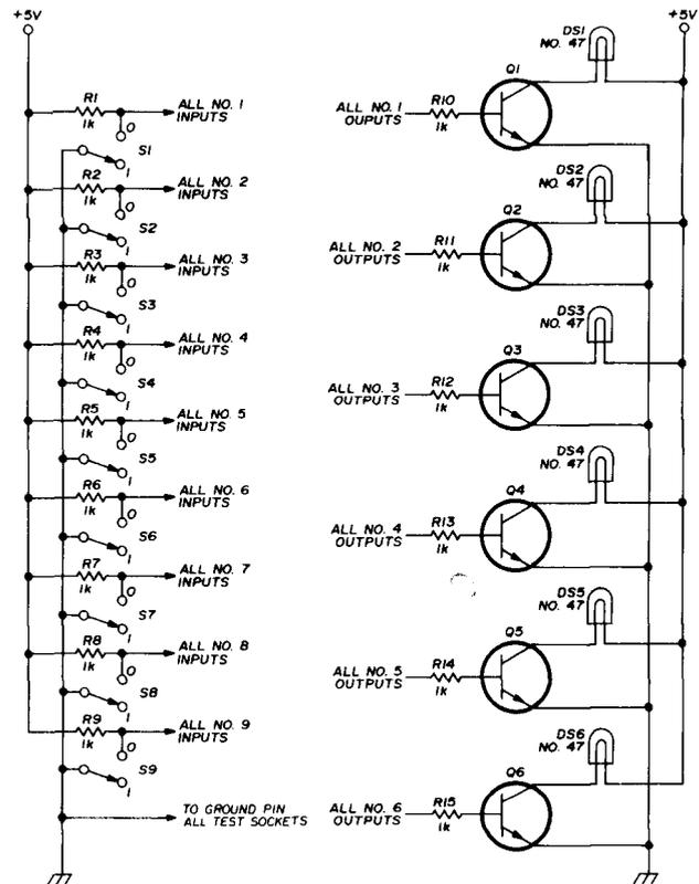
fig. 1. Schematic of the IC tester.
