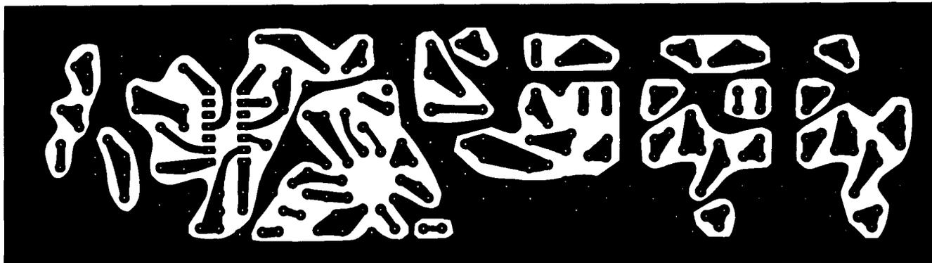
fig. 8. Printed-circuit board layout for the rf amplifier and mixer (left side of board) and the detector and audio filter. Board is 7-7/8" (20cm) long by 2-1/8" (5.4cm) wide.
