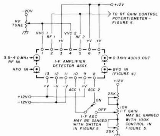
fig. 7. Sophisticated operating mode for the i-f/detector module.
