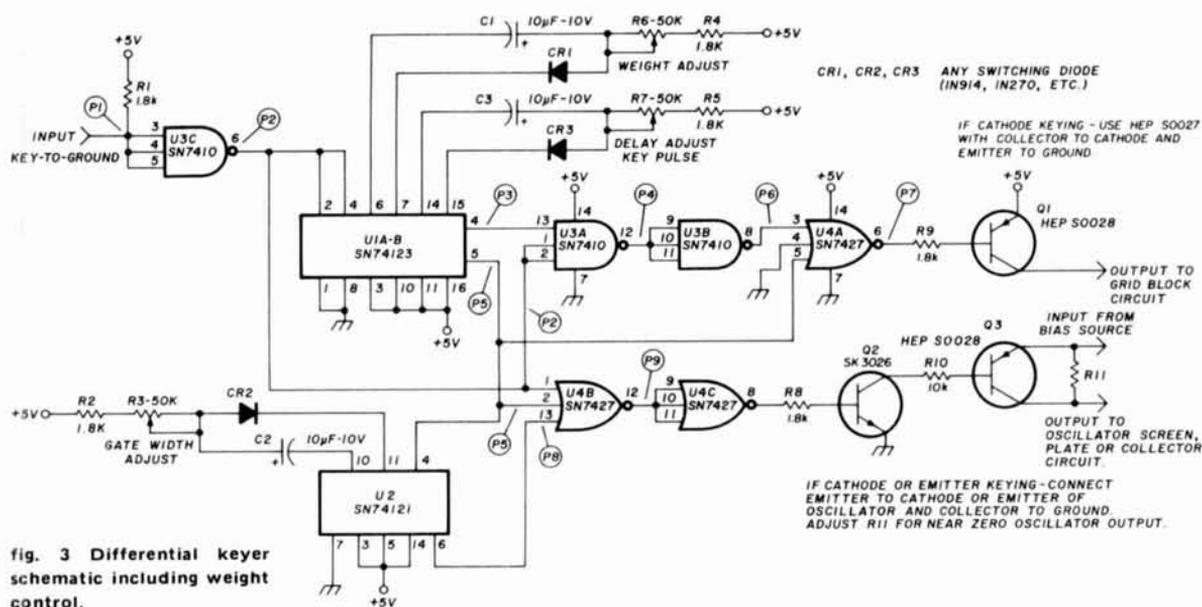
fig. 3 Differential keyer schematic including weight control.
