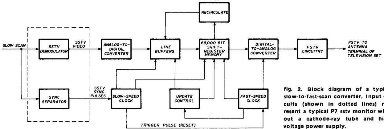
fig. 2. Block diagram of a typical slow-to-fast-scan converter. Input circuits (shown in dotted lines) represent a typical P7 sstv monitor without a cathode-ray tube and high-voltage power supply.
