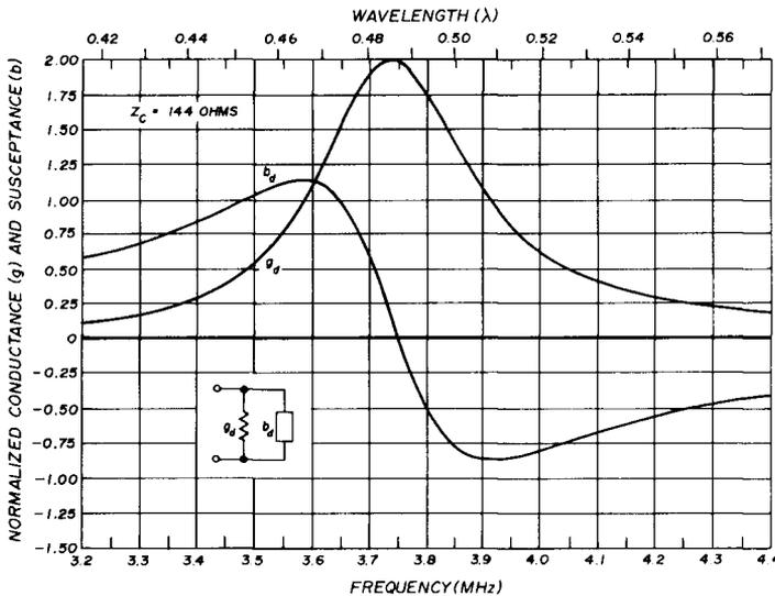
fig. 3. For ease of calculation, the impedance values of fig. 2 have been converted to admittance and plotted in terms of normalized conductance,  $g$ , and susceptance,  $b$ . Feedline impedance of 144 ohms yields optimum bandwidth, as discussed in the text.
