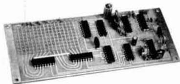
With the new CW ID kit offered by VHF Engineering, you can build a complete identifier for commercial or amateur repeaters in about one evening. The CW ID kit uses high-grade components and comes complete with a drilled epoxy-glass circuit board and programming diodes.
