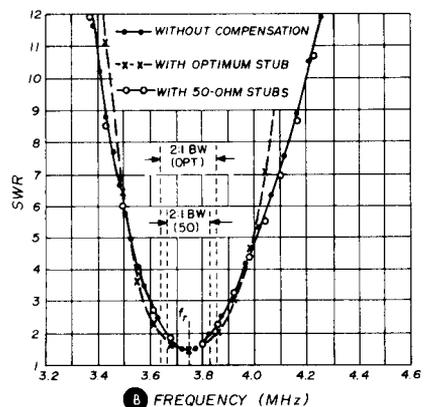
fig. 9. Swr vs frequency for compensated and uncompensated dipoles fed with 100-ohm (A) and 50-ohm (B) feedlines.
