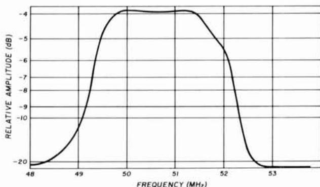
fig. 2. X-Y recorder plot of filter response. Filter insertion loss pushes down the peak of the curve allowing skirts to show out-of-band values of signals passed.
