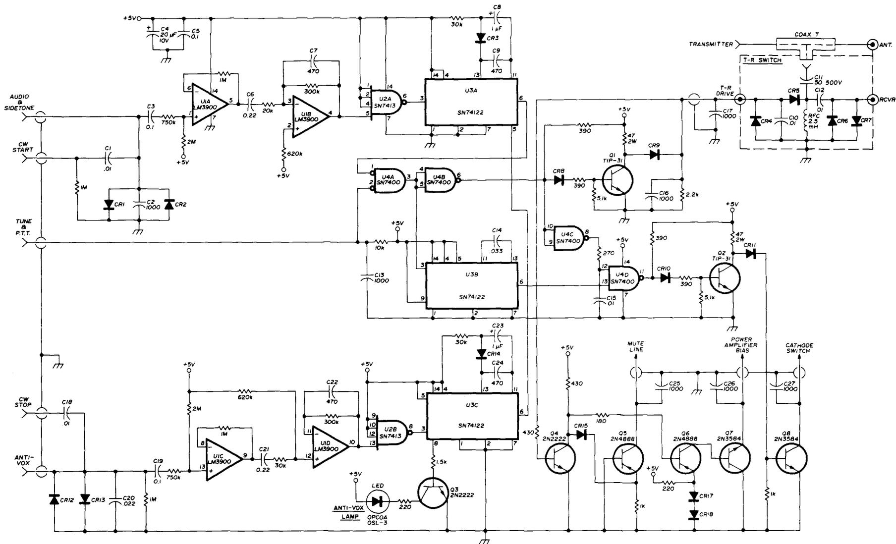
fig. 1. Syllabic vox and CW break-in system schematic for use with the Drake T-4XB and R-4B transmitter and receiver. Circuit provides instantaneous speech communication without conventional voxA relays. Diodes CR4, CR5, CR6, CR7, CR9 and CR11 are 1N4004 or equivalent; all other diodes are 1N914 or equivalent. The rf choke is a 2.5 mH transmitting type (100 mA). All resistors are 1/2 watt, 10% unless otherwise specified.
