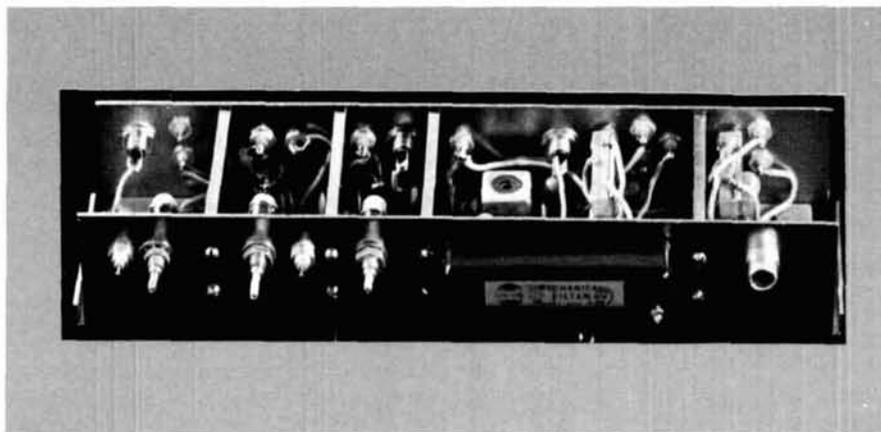
High-performance i-f/detector receiver module, cover removed. Enclosure is an LMB 850 box. Rf input is at right; audio output at left.
