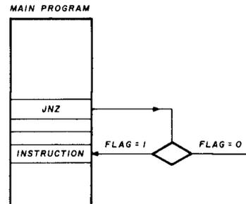
fig. 1. The JNZ instruction. If the zero flag is at logic 1, the instruction is ignored and program control passes to the following instruction.
