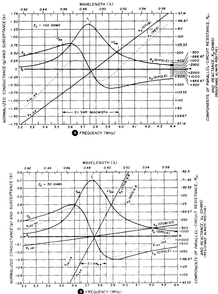
fig. 8. Normalized admittance parameters for uncompensated and compensated half-wavelength dipoles fed with 100-ohm (A) and 50-ohm (B) feedlines. Conductance,  $g_d$ , and susceptance,  $b_d$ , are for the uncompensated case. Stub susceptance,  $b_s$ , and resultant susceptance,  $b_{res}$ , are also shown. The optimum stub susceptance for the 50-ohm case ( $b_s = 6.8$  ohms) gives maximum swr bandwidth.
