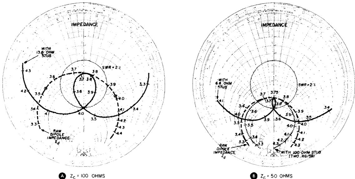
**fig. 10. Smith chart plots of normalized impedance for compensated and uncompensated half-wavelength dipoles fed with 100-ohm (A) and 50-ohm (B) feedlines. Optimum stub impedance for 100 ohm case is 13.8 ohms; optimum stub impedance for 50-ohm feedlines is 6.8 ohms.**
