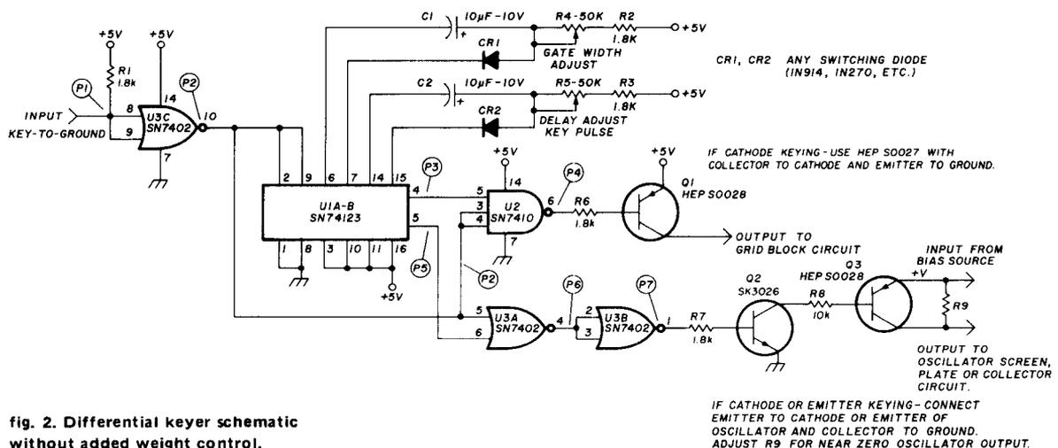
fig. 2. Differential keyer schematic without added weight control.
