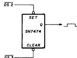
fig. 2. SN7474 flip-flop used as a monostable multivibrator.
