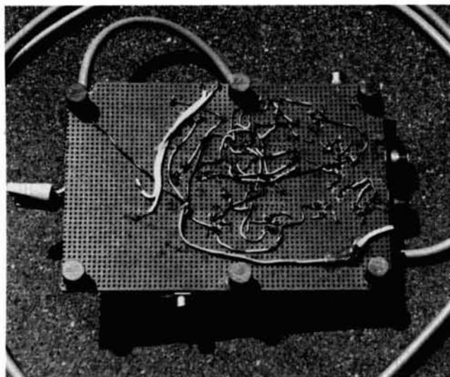
Underside of perf board showing point-to-point wiring.
