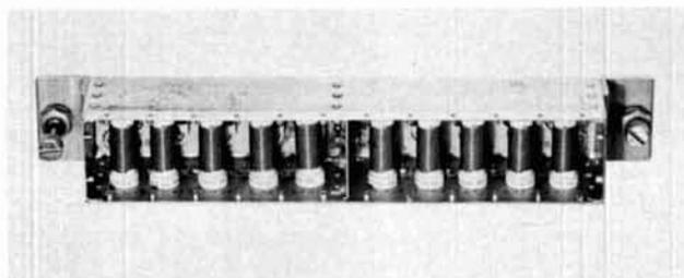
Inside the 50-MHz bandpass filter showing coil arrangement and center shield. (Photo courtesy Paul Ireland).
