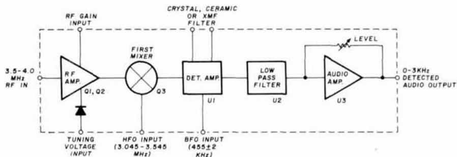
fig. 1. Block diagram, high-performance i-f/detector receiver module.
