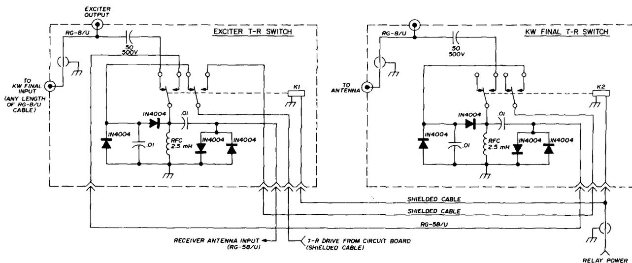
fig. 3. T-R switch schematic for use with kilowatt final amplifiers. Suggested relays are Potter & Brumfield type KT-11D. Each T-R enclosure should be mounted to each output by rigid coaxial connectors. A bud type CU-234 utility box is suggested for each T-R switch.
