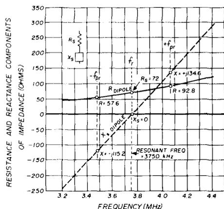
fig. 2. The series resistance,  $R_s$  and reactance,  $X_s$  components of uncompensated dipole impedance versus frequency. Values shown here are for a half-wavelength thin-wire dipole in free space.<sup>11</sup>
