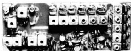
Top view of the completed 2-meter fm exciter showing clean layout of parts without overcrowding.
