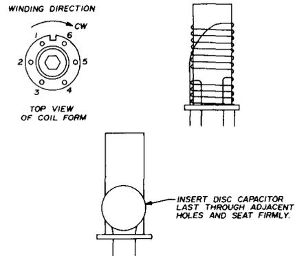
fig. 3 Diagram for winding coils (exaggerated for clarity). The number of turns for all coils is shown in the schematic. All turns are close spaced; winding direction is extremely important.
