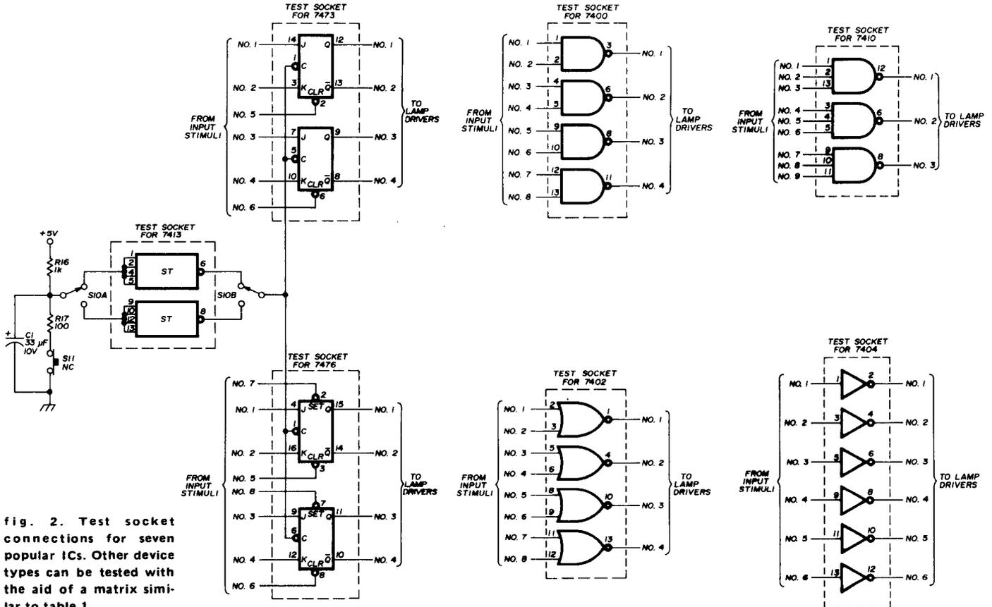
fig. 2. Test socket connections for seven popular ICs. Other device types can be tested with the aid of a matrix similar to table 1.
