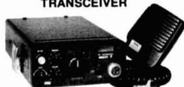
23 xtl chans. (external VFO). NBFM. 10W power out. Sensitive, double-conversion receiver. Mobile. 13.5VDC
