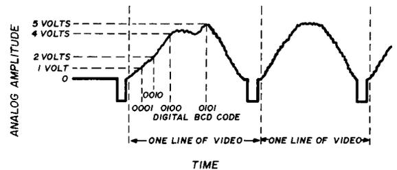
fig. 3. Each line of slow-scan video voltage is sampled at a periodic rate (approximately 256 times per line), which results in 256 digital words per line, each containing four bits of gray-code information.
