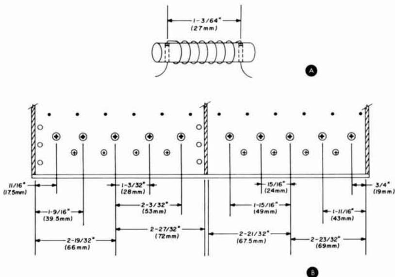
fig. 4. Coil construction details (A) and side view of filter box showing coil spacing (B). Enclosure dimensions are 2-1/8 inches (54mm) deep and 1-7/8 inches (47.6mm) across opening.
