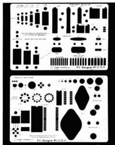
The new *PC Designer* template set has been updated to include additional, frequently used component packages and mounting patterns for printed-circuit layouts and assembly drawings. All patterns conform to guidelines established by Mil-Std 275C and The Institute of Printed Circuits bulletin CM-770. Component mounting patterns are on grid centers which enable the designer to design for automatic insertion assembly equipment.
