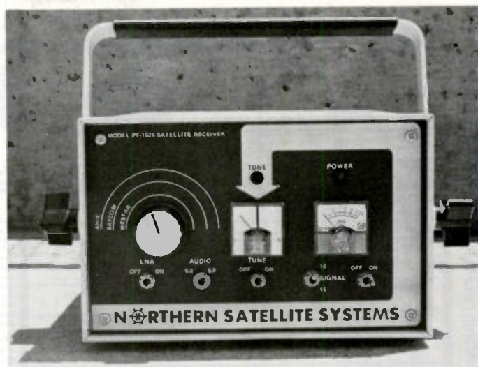
Photo K. Private terminal receiver designed initially for Canadian "backwoods terminals" features continuous tuning dial, tuning meter (with afc on and off switch), and selectable aural subcarriers. Unit (PT-1024) is manufactured by Satco, in Lewisville, Texas.
