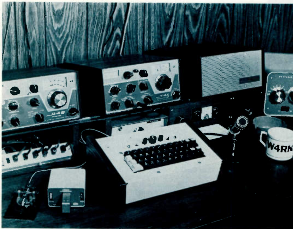
This is a view of the code typewriter amidst other CW-making equipment in the W4RNL shack. The photo also shows clearly how the use of wood end pieces will obtain the slope needed for the keyboard. To enjoy CW, everything on the operating table (including the coffee cup and ashtray) is needed except the mike. The 25-year-old J-38 and the Codax keyer are used often in an attempt to send CW as perfectly as does the typewriter.
