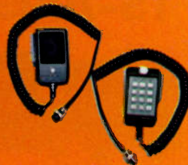
MC-45 Touch-Tone (with automatic transmit) microphone.
