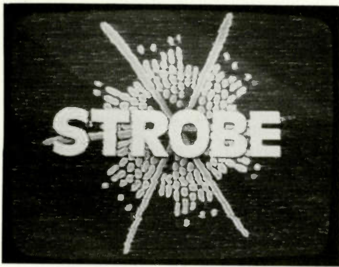
Photo J. Six-foot antenna pictures from WESTAR I. This picture exhibits noise (known in the trade as "sparklies"); LNA in use when the picture was taken was a 1.5-dB noise level unit, about 0.5 dB too "high" for noise-free pictures.
