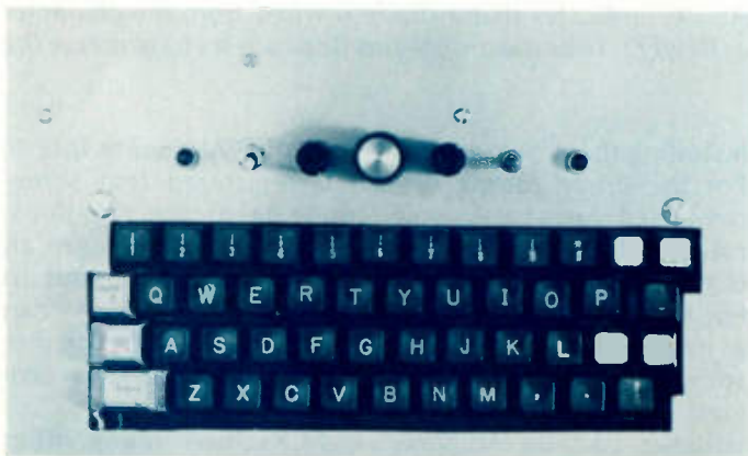
This is a close-up top view of the code typewriter. The controls above the keyboard are, from left to right, the ac pilot light, power switch, volume control, speed control, tone control, tune-up switch, and tune-up pilot light. Keys with white squares were labeled by using adhesive address labels with a transparent tape cover; all were typed and then cut to fit the keys. The DOT and DASH keys have had their internal resistors removed.
