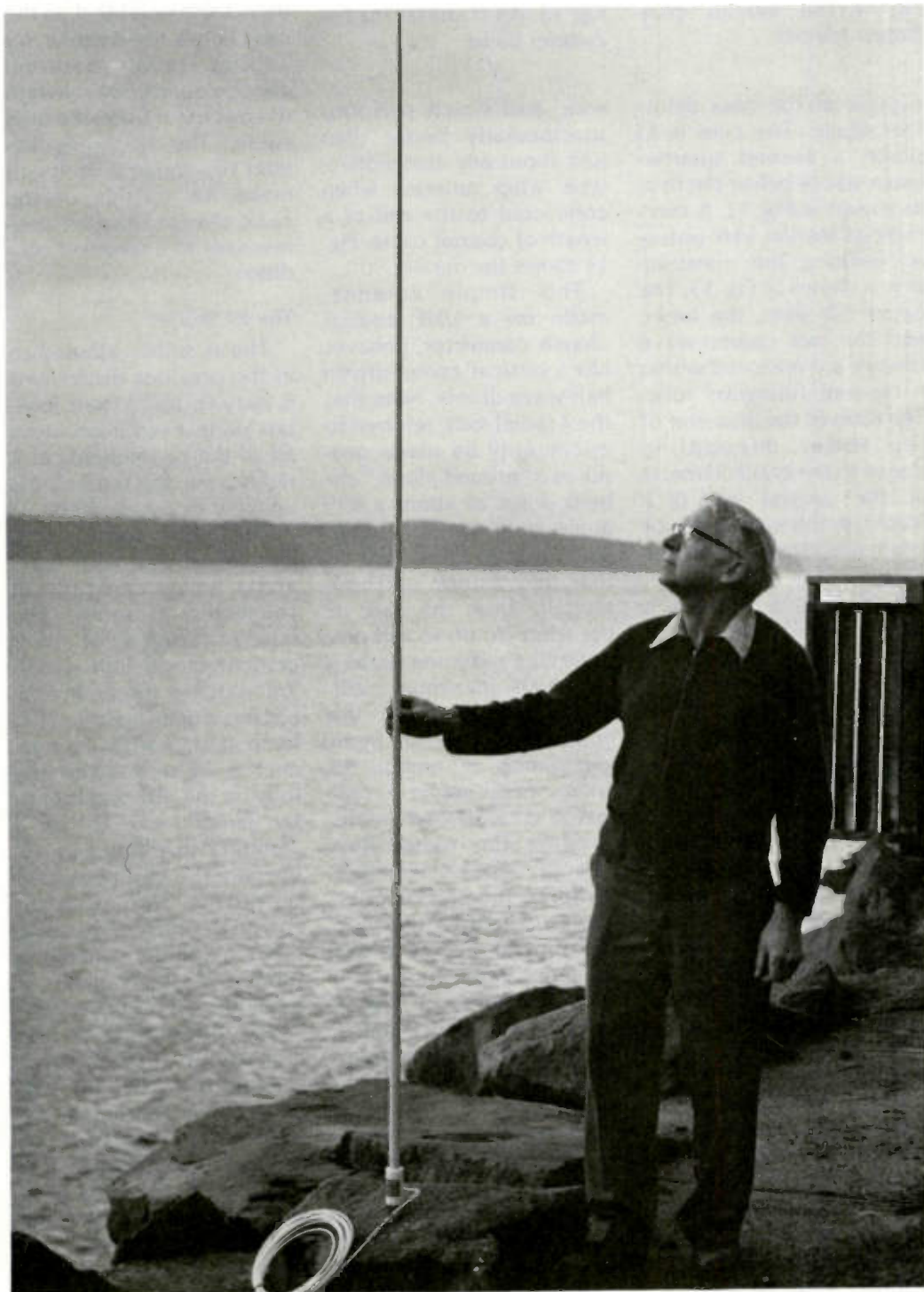
Fig. 13. Commercial VHF version of marine antenna shown in Fig. 12. Here, the author provides temporary (and decoupled) support.
