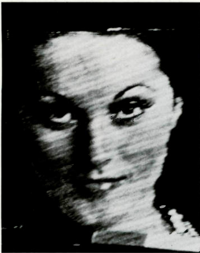
Photo 3. SSTV picture digitized to 256 pixels with 16 gray levels.
