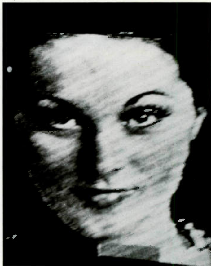
Photo 4. SSTV picture digitized to 128 pixels with 64 gray levels.
