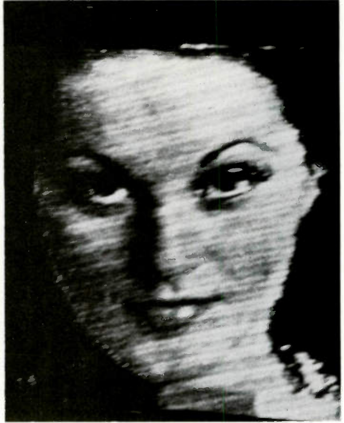
Photo 2. SSTV picture digitized to 128 pixels with 16 gray levels.
