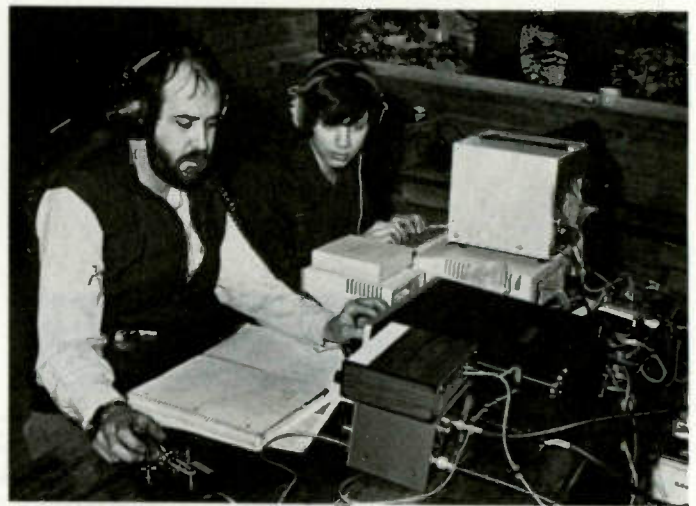
The Novice/Tech station of K8EMY. This station was run totally on dc using an auto battery charged by a small gas generator. At left is Ron Headley WD8QAZ and at right is Ron Wexler KA8CBQ. Also pictured is a minicomputer lent to the club by "Computerland." This Apple was used to log contacts and keep track of points. The antenna for the station was a mobile one located on WD8QAZ's Honda.
