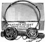
The world famous TRIMM Featherweight. Recognized as a leading quality headset. Weighs 4 1/2 oz. complete with two units, 5-foot moistureproof wear-resisting cord. Bakelite shell and cap. Magnet of highest quality cobalt steel alloy. Pole pieces of finest magnetic iron. Coils especially impregnated. A custom-built phone throughout. Standard resistances.
