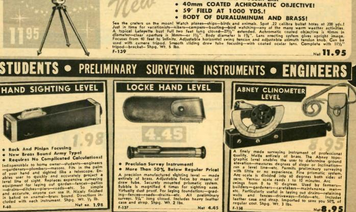
A precision manufactured sighting level — made entirely of brass. Adjustable focus by means of draw tube. Securely mounted prismetic system. Bubble is magnified 4 times for sighting ease. Virtually dust proof. For laying foundations—grad-virtually dust proof. For laying foundations—grad-ing—fences—roads—drains—etc. All preliminary surveys. 514" long closed. Includes heavy leather case and strap. Shpg. Wt. 2 lbs. F-137 Net 4.65
