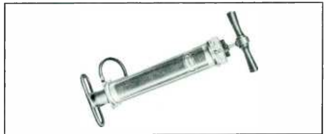
Type No. 30-150 DEHYDRATOR, hand pump consists of blue indicating gel, and will pressurize up to 1000 ft. of 7/8" or 250 ft. of 1 1/8" Spir-O-line. (Part No. 099 0517 00).
