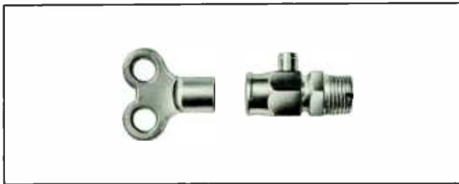
Type No. 33-150 BLEEDER VALVE, with key has \frac{1}{8} " IPS male thread used wherever necessary when purging transmission line. (NPN).
