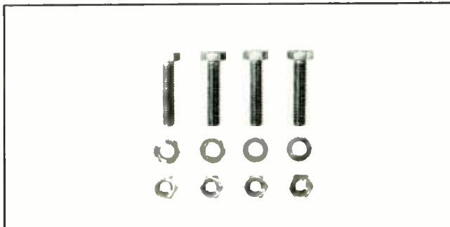
TYPE NO. 315-825 (NPN) — Hardware set for 1\frac{3}{8} " flanges. Consists of 4 ea. stainless steel bolts, nuts and lockwashers, \frac{5}{8} "-18 x 1\frac{1}{2} " lg. Weight: 3\frac{1}{2} oz.
