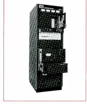
Front view of FM-1.5A Transmitter illustrates modular slide out construction.
