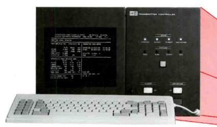
Five plug-in cards for the optional microprocessor system are housed behind hinged Transmitter Controller panel. To left is CRT monitor for bar-graph and tabular information read out display, and keyboard for message programming and display page access.
