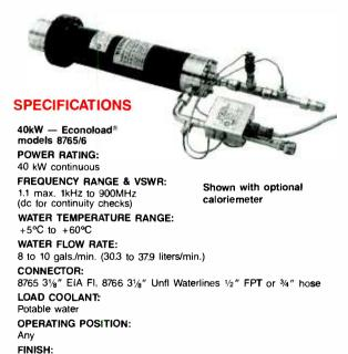
FINISH: Semi-Gloss black enamel NOMINAL SIZE:  $19^{1/2''} \times 3^{1/2''}$  dia. (495 × 90mm). Input Flg. 5<sup>13</sup>/<sub>16</sub>" dia. (132mm) WEIGHT: 8755 13 lbs. (5.9kg), 8756 12<sup>1</sup>/<sub>2</sub> lbs. (5.7kg)
