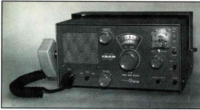
Tram's name on any piece of early CB equipment meant it was something special. Here's the company's Model TR-70C transceiver from about 1963. During the 1970's, they made spectacular CB sideband equipment. (Courtesy Tom Kneitel)
