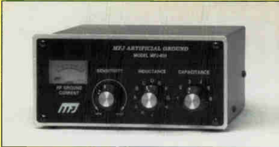
The MFJ-931, Artificial RF Ground device is ideal for apartment dwellers who live on upper floors where no earth ground is possible. (Photo Courtesy MFJ Enterprises)
