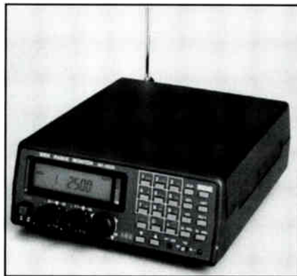
This wide-coverage scanner from AOR offers not only the VHF and UHF scanner bands, but also extended coverage of 800 and 900 MHz for newer radio systems.
