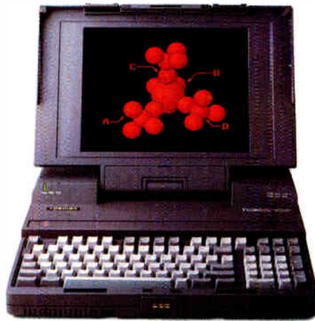
T5200: 20MHz 80386 processor, 2 internal IBM compatible expansion slots, 40 or 100MB hard disk, VGA display with external VGA monitor port, 2MB RAM expandable to 8MB.
