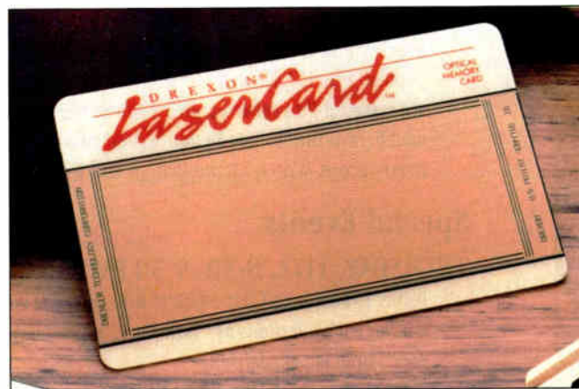
Photo 9: Drexler's wallet-size LaserCard contains a 35-mm strip that can permanently store several megabytes of data. Its current use is storing medical and insurance data.
