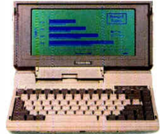
TL200FB: 9.8 pounds, 9.54MHz 80C86, 1MB RAM, 2 720KB 3 1/2" floppy drives, removable/rechargeable battery pack.
