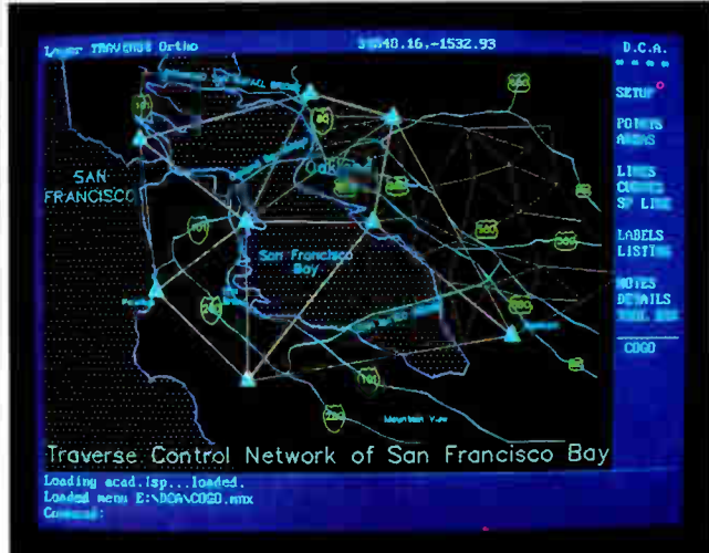
The Surveyor, a coordinate geometry program for surveyors and civil engineers, can handle sites as large as San Francisco.
