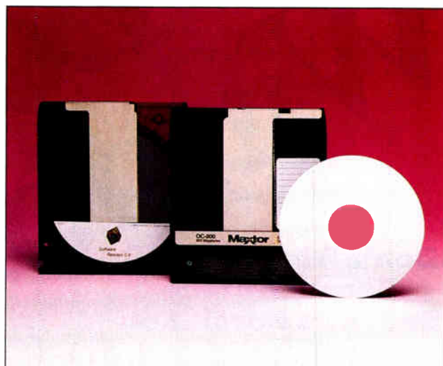
Photo 6: Optical disks are known for their extremely large capacities. Shown here are a WORM (write once, read many times) disk, a CD-ROM, and a magneto-optical erasable NeXT cartridge. You can store almost a gigabyte of information on the WORM disk, 550 megabytes on the CD-ROM, and 256 megabytes per side on the NeXT disk.
