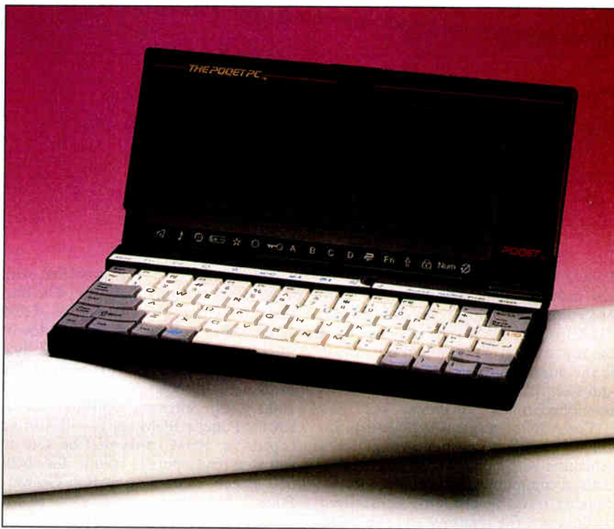
Photo 1: The Poqet PC, shown unfolded. The small nonbacklit LCD screen can display 25 rows of 80 columns and CGA-compatible graphics. The keyboard features 77 keys, with each key measuring about one-half inch square, and has an embedded numeric keypad.
