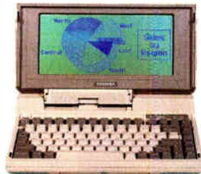
T1200HB: 10.8 lbs, 9.54MHz 80C86, 20MB hard disk, 1MB RAM, includes 384KB LIM-EMS. Removable/rechargeable battery pack.
