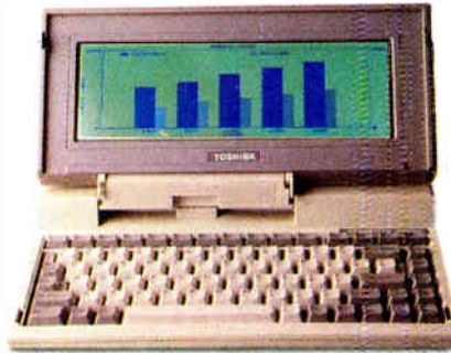
T1000: 6.4 lbs, 4.77MHz 80C88, 512KB RAM expandable to 1.2MB. MS-DOS in ROM, 720KB 3 1/2" diskette drive. Built-in RGB, parallel, serial and external drive ports.
