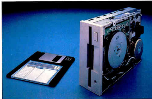
Photo 8: A "floptical" disk is a 3½-inch floppy disk that uses optical and magnetic recording technologies and can hold 20 to 25 megabytes.
