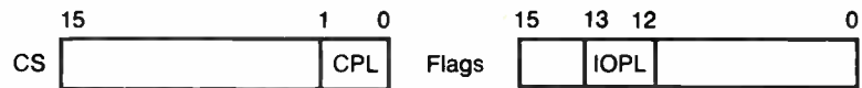
Figure 3: The CPL is located in the last two bits of the code segment's selector. The IOPL is found in the program's flags. You can modify the IOPL only when CPL=0; you can execute sensitive instructions only if CPL <= IOPL.
