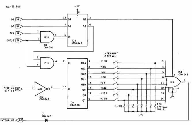
**Figure 1:** Schematic diagram of the clock hardware and its connection to the Elf II bus. The clocked interrupts are developed from system-timing signals to alternate with interrupts from the video display; neither will interrupt the other while it is being serviced by the processor. A set of DIP switches allows the user to select a division factor so that interrupts can occur at regular intervals from about two per second to one per minute.
