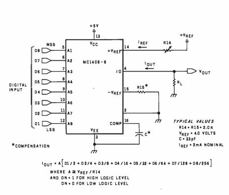
Figure 3: A circuit employing the Motorola MC1408-8, a typical 8-bit current-output monolithic multiplying D/A converter. This integrated circuit contains an R-2R network like the one in figure 2, plus additional current-switching logic.
