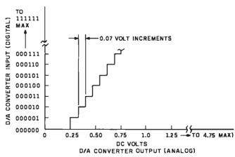
**Figure 7:** DAC output as a function of digital input. The output should increase monotonically as shown.
