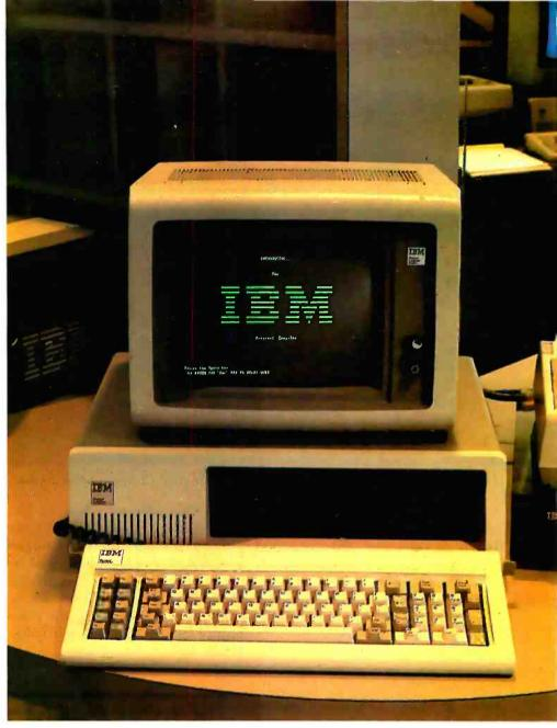
Photo 2: The IBM Personal Computer System with the IBM Monochrome Display.
