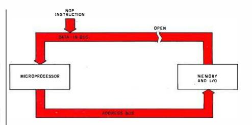
**Figure 2:** One method for generating signals for signature analysis. The data-in bus is opened, and a NOP instruction is forced on the bus. This causes the processor to constantly increment the program counter, so that a stream of values appears on each address line. Interrupts should be disabled.
