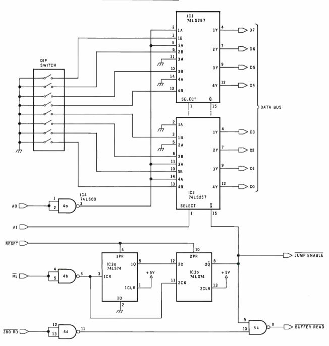
**Figure 1:** Schematic diagram of the circuit used to force Z80 starting addresses to any of 256 memory pages. IC1 and IC2 are threestate multiplexers that pass the address set by the switches when the proper combination of reset signals occurs.
