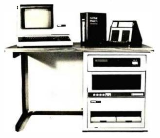
**CI-MWS23-MB** — LSI 11/23 computer workstation. LSI 11/23 CPU, MMU, 256KB Memory, power supply, in 16 slot rack mountable chassis. CRT terminal. 10 mega byte cartridge disk system. 4 port serial I/O. Desktop workstation ..... **\$11,995.00**
