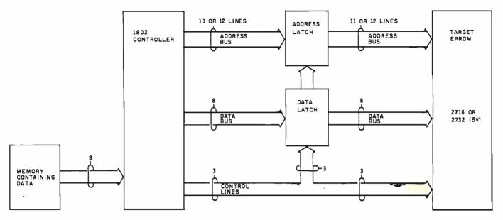
**Figure 1:** A block diagram of the EPROM-programmer system. The 1802 microprocessor provides address and data signals to latches, then, through the use of various control signals, releases the information from the latches at the proper time to program the EPROM.
