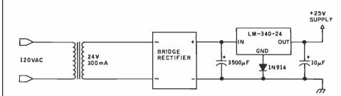
Figure 2c: A + 25-V supply provides programming voltage. A + 24-V regulator is used in conjunction with a diode to produce +24.6 V—well within the  $\pm 1$ -V tolerance specified by EPROM manufacturers.
