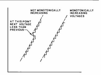
**Figure 13:** For digital inputs from 0 to 63, the output from the DAC should increase monotonically (as in the curve on the right). Otherwise, the A/D circuit will give invalid readings for analog values in that voltage region.
