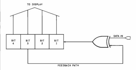
**Figure 1:** A simplified version of a signature analyzer. In this scaled-down unit, only four bits are used in a shift register (as opposed to 16), and a simple exclusive-OR gate is used in place of the adder. Each bit of the incoming data stream is fed back to the exclusive-OR gate as it reaches the third position in the shift register.
