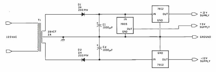
Figure 1: Simple and inexpensive power supply for the Z80 Starter Kit. It will provide +5 V at 1 A and  $\pm 12$  V at 200 to 300 m A for the Z80 Starter Kit and user circuitry. Parts used include: T1: 120 VAC primary, 28 VAC center-tapped secondary, 2 A;D1,D2: 3 A, 200 V PIV silicon diodes; C1,C2: 1000  $\mu$ F, 50 V electrolytic capacitors (note polarity carefully); 7805: +5 V, 1.5 A voltage regulator; 7812: +12 V, 1.0 A voltage regulator; 7912: -12 V, 1.0 A voltage regulator.
