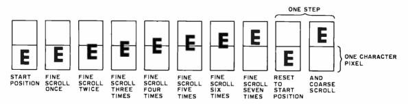
**Figure 2:** In order to achieve fine scrolling over the entire display screen, a combination of fine and coarse scrolling is used. After the seventh fine scroll is performed, the fine-scroll register is reset and a coarse scroll is performed.
