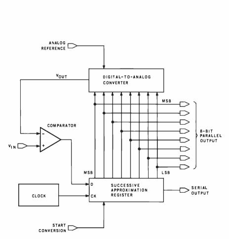
**Figure 11:** Block diagram of a typical 8-bit successive-approximation A/D-conversion system.
