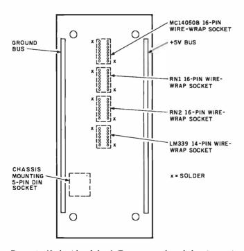
**Figure 9:** Underside of the A/D prototype board showing positions of ground and +5-V buses and solder points for the wirewrap sockets.
