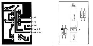
Figure 2: Interface etching, drilling, and component layout. A printed-circuit card of the proper size (the figure is actual size) will fit easily in the controller's case, although other construction techniques may work as well. Note the orientation of pin 1 on each of the integrated circuits.
