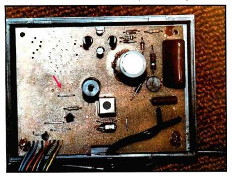
**Photo 1:** The standard BSR command console. This unit is exactly the same as the ultrasonic version but does not have the 40-kHz transducer and amplifier. The arrow points to a jumper at the input of the custom LSI controller integrated circuit developed by BSR. This is the input that can accept serial information from a computer. (Photo courtesy Dan Thompson)
