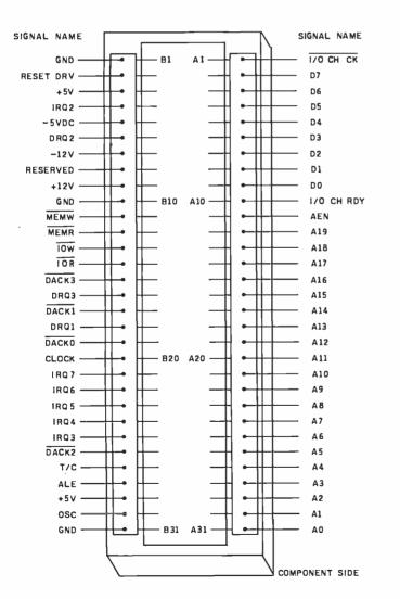
**Figure 4:** Electrical signals on the IBM System Board I/O Channel (expansion slot). See table 3 for signal descriptions.
