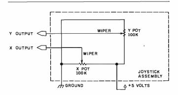
**Figure 5:** Joystick schematic. Two 100-k-ohm potentiometers are connected to ground and +5 V. Each wiper outputs a voltage of 0 to 5 V depending upon the joystick position along the X and Y axes.
