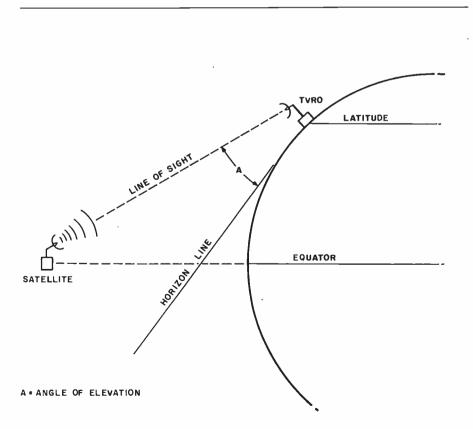
**Figure 2:** Elevation angle for the antenna is measured from the horizon (0 degrees) to straight up (90 degrees).
