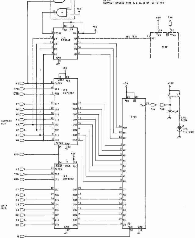
**Figure 2a**: A schematic diagram of the EPROM programmer, which illustrates the use of one 1852 8-bit latch (IC4) to hold the data that will be programmed into the EPROM. An 1852 and the combination of a 4042 latch and a 4011 NAND device are used to hold up to 12 address bits.
