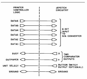
**Figure 3:** Line-printer lines used in the A/D circuit. Six output lines transmit a digital value to the DAC. Two input lines read the comparator values. One optional input line allows checking the button switch on a joystick.
