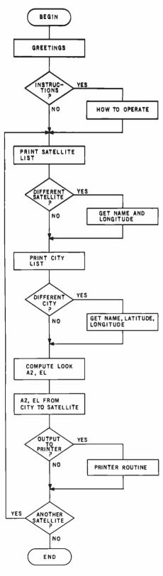
Figure 3: A flowchart showing organization and operation of the GEOSAT program.
