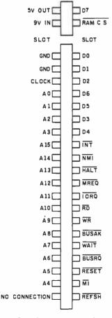
**Figure 1:** Signal pinouts on the ZX-80 edge connector as seen from the rear.
