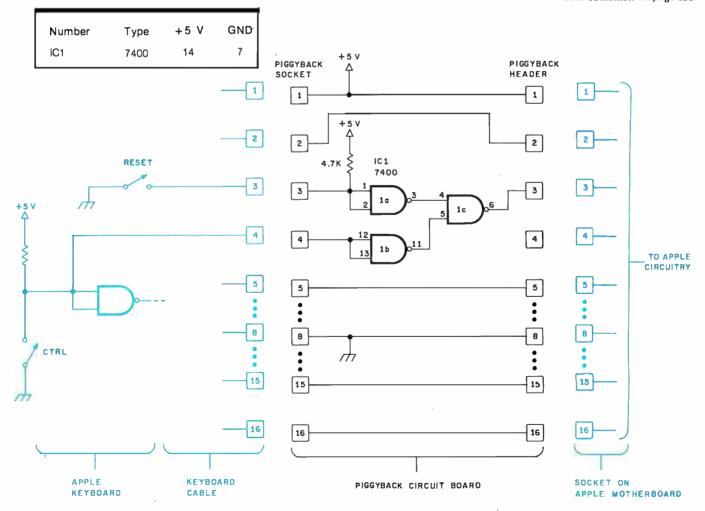
**Figure 1:** Schematic diagram of the control-plus-reset modification to the Apple II computer. One connection from the control key to pin 4 of the keyboard circuit board is shown in this diagram and figure 2. The cable from the Apple keyboard plugs into the pig-gyback board socket, and the piggyback board header (on the other side of the printed-circuit board) plugs into the socket on the main Apple board (the motherboard). Pins not shown have connections similar to pin 5.
