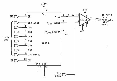
Figure 10: A software-driven 8-bit A/D converter.
