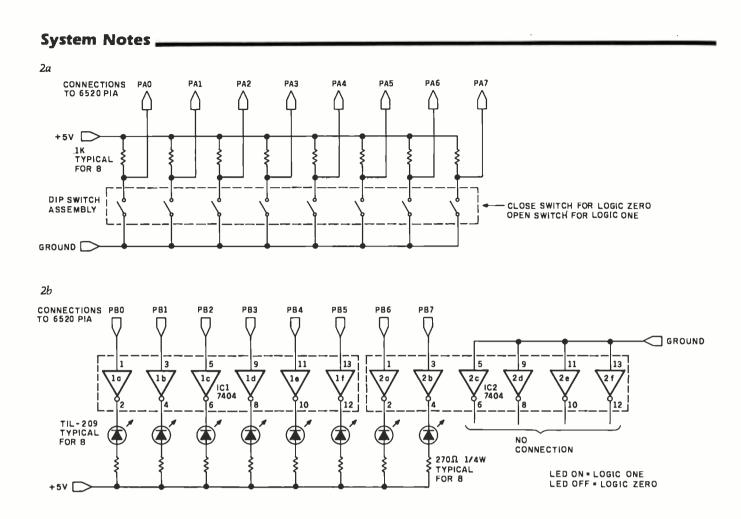
Figure 2: Controls and indicators for testing the circuit of figure 1. Figure 2a diagrams a method for manually setting the logic conditions on one port of the 6520. Figure 2b shows a circuit that indicates the logic state of each bit in one port of the 6520.
