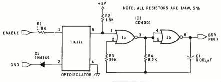
Figure 1: Schematic diagram of the serial interface circuit. The ENABLE signal may be originated by a computer's RS-232 port or from a parallel port driven by the appropriate software. The optoisolator is used to isolate the controller from the computer (the controller's ground "floats" at power-line voltage). The oscillator made from IC1 is designed to produce a
