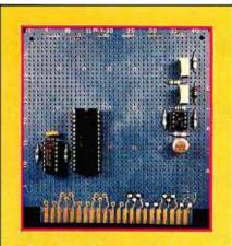
Photo 2: Prototype of the analogto-digital converter system of figure 13, which uses the Analog Devices AD7581 integrated analog-to-digital converter.
