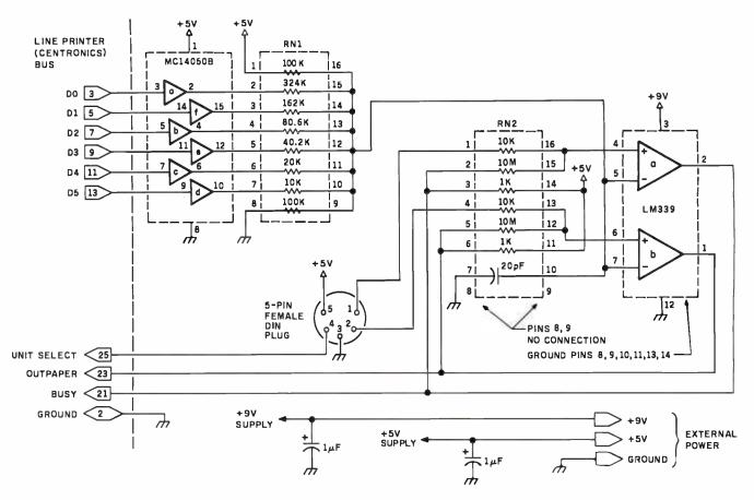
Figure 4: Detailed logic diagram of the A/D circuit. Power is supplied by a 9-V transistor battery and a 5-V power supply.
