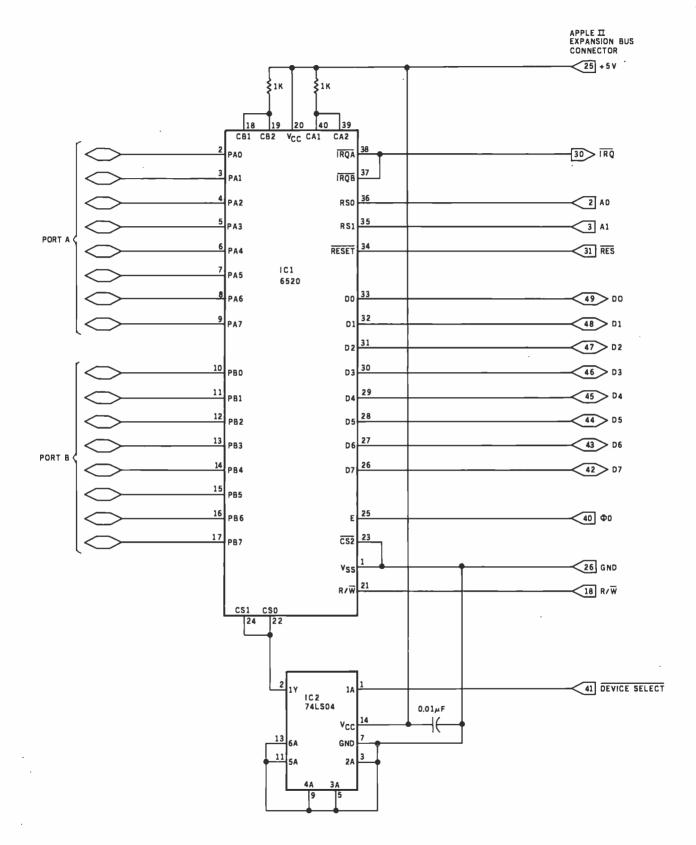
**Figure 1:** Interfacing an Apple II to a 6520 peripheral interface adapter. The active-low select line of the 6520 is tied to ground while both active-high select lines are connected via an inverter to Device Select (an active-low signal generated by the Apple II that enables one of its eight peripheral positions).
