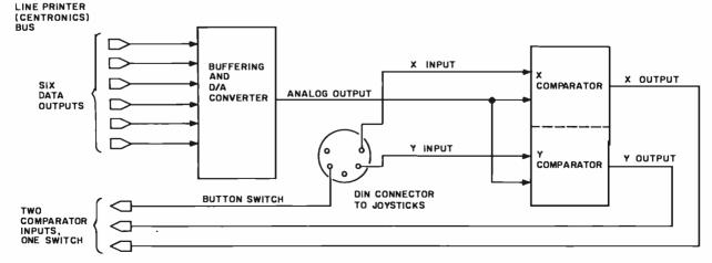
**Figure 1:** Block diagram of the A/D circuit. The DAC is driven by outputs from the line-printer port. Its output goes into two comparators, one comparing the DAC voltage with the X channel, and the second comparing the DAC voltage with the Y channel. The comparator outputs are fed back into the line-printer port.
