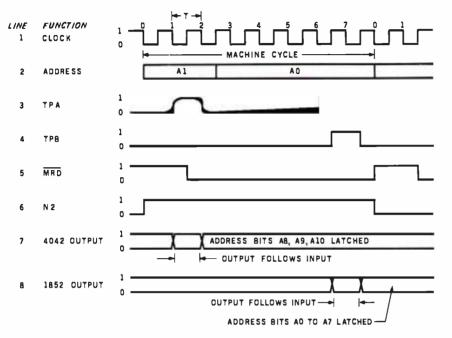
**Figure 4:** The 1802 timing diagram is broken into eight T-cycles. A machine cycle can be either a fetch or an execute cycle; the diagram here shows the execute phase and the timing relationship of the control signals.
