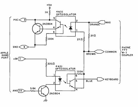
**Figure 1:** A schematic diagram of the Apple/M-1 coupler interface. The circuit uses optical isolators to convert the coupler's 60-mA current loop to the TTL levels required by the Apple game-paddle interface.
