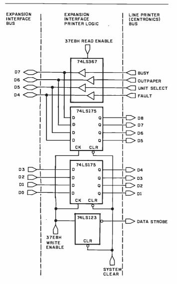
**Figure 2:** Model I line-printer controller. Two 4-bit registers strobe in the 8 bits of the character to be printed. At the same time, the one-shot is set to allow the output line-printer electronics to strobe in the data from the register. Four status lines are gated to the computer's data bus on a read.
