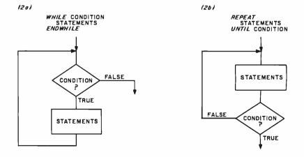
**Figure 2:** Flowchart symbols used to represent the WHILE...ENDWHILE (figure 2a) and REPEAT...UNTIL (figure 2b) programming constructs.
