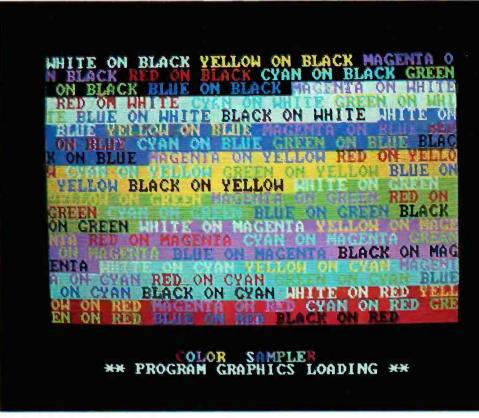
**Photo 8:** An example showing the independence of foreground and background colors when using the text mode of the color/graphics adapter board.
