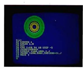
Photo 7: An example of combining text and graphics on the same video screen. The program shown, when run, generates the circular image just above it.
