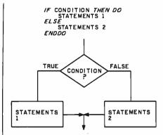
**Figure 1:** Flowchart symbols used to represent the IF...THEN...ELSE...END-DO programming construct that is important to structured programming.
