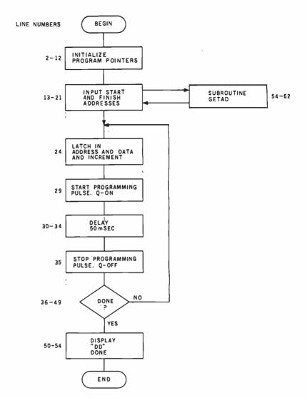
**Figure 5:** A flowchart of the program for controlling the 1802. The numbers to the left of the box symbols correspond to program line numbers.
