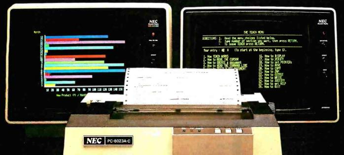
The impressive new NEC dot matrix printer. Parallel interface, 100 cps, 2K buffer, pin or friction feed. Stunning performance and versatility in the hottest new peripheral of the year.
