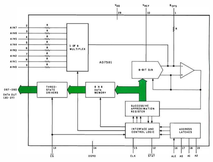
Figure 12: Functional block diagram of the Analog Devices AD7581 A/D converter.
