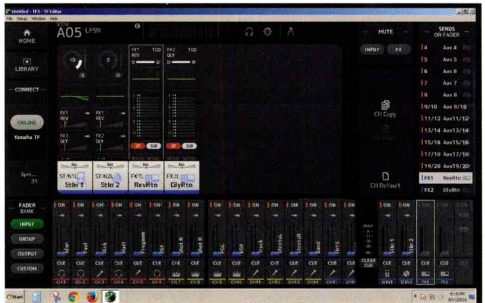
TF Editor puts TF3 programming and control on a Mac or PC.
