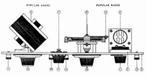
Fig. 2. A top view of the parts and panel layout of the receiver. The major components from left to right: The Haynes variometer, rheostat, tuning capacitor, and the second rheostat above the tube socket.
