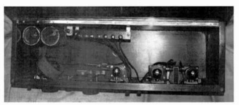
Figure 3. A view of the internal workings of the Haynes-Griffin Dx receiver showing the layout of the components.
