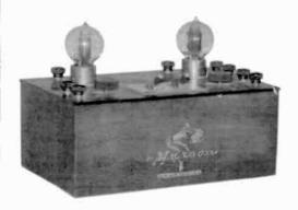
MAGNAVOX TYPE AC-2, MODEL C AMPLIFIER - This 2-tube amplifier, found locally, is signed "Chas. H. Humphreys - Macon, GA" and is dated 1922. The tube sockets have double bayonet slots for either Type 01-A tubes or WE tennis ball types as shown. (Joseph G. Jackson - Macon, GA)
