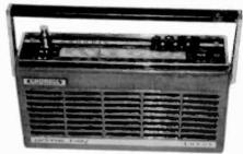
**GRUNDIG PRIMA-BOY LUXUS** – This is a fine transistor portable of the late 1960s. It has no AC power cord and operates only on batteries. It receives the following European ranges: UKW, KW, MW, and 49m. (Erwin Macho – Vienna, Austria)
