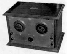
1924 Marconiphone Model VI, a 1-valve battery receiver for headphone use, tuning from 300 M to 4600 M in six bands.
