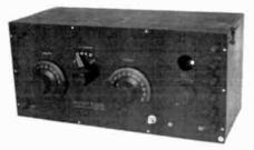
Figure 2. Closeup of the 1-tube receiver section. (From the John V. Terrey collection.)
