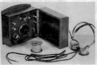
HOME-BREW CRYSTAL SET – I designed and bullt this catwhisker type crystal set using old antique parts. Housed in an old meter case, it works very well with a pair of Western Electric headphones. (Joseph Wood – Hodgkins, IL)
