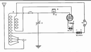
Fig. 1. The schematic diagram for the Haynes-designed 1-tube regenerative receiver. Note the "Load" connections used to extend the set's tuning range.
