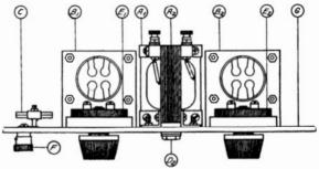
Fig. 4. A top view of the amplifier layout. The binding posts are located on the left side of the panel to allow connections to the receiver.
