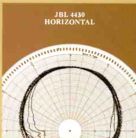
Polar response of a 4430 studio monitor:
