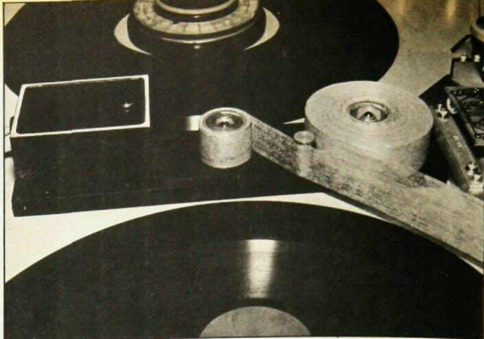
Motorized tape cleaner. The cleaner wipes loose oxide and foreign matter before the tape enters the head assembly. The tape cleaner runs only when the duplicator is in the RUN mode. One roll of tape has an approximate running time of 250 hours. The tape cleaner is used with either the Master or the Slave.
