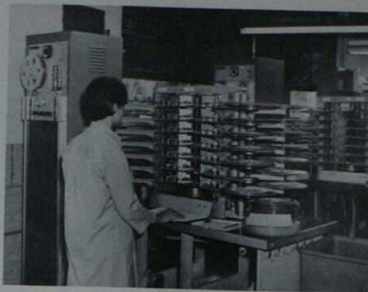
DUBBINGS ELECTRONICS has added four new duplicators to its operation in Copiague, New York. Each of the four units incorporates 14 slaves. The tape master moves past the capstan at 120 ips, while each of the slaves operates at a 30 ips speed.
