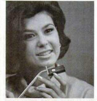
INTEGRATED CIRCUIT comes to the phonograph in the 1968 RCA Victor line. The IC, under the cap in the tone arm, acts as a pre-amp and is said to reduce the possibility of distor-
