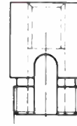
Thread Adapter with Cable Outlet M 17 x 1-5/8" Female and for mounting on panels up to 7 MM
