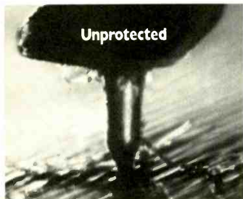
Magnification shows the record vinyl wearing away.
