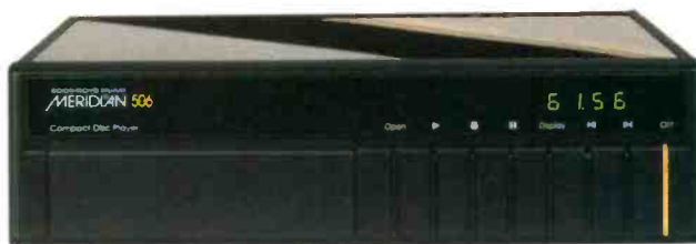
Meridian's elegant Model 506 player ($1,495) uses a nonmagnetic disc-clamping mechanism to minimize vibration and has both optical and coaxial digital outputs. A Meridian System Remote is included.
