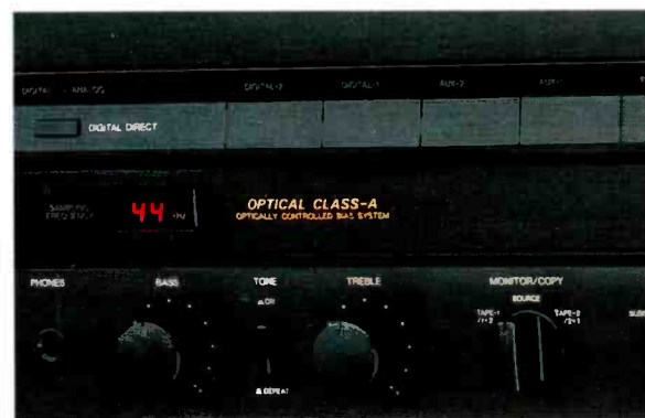
The conversion circuits in Denon's PMA-1520 integrated amplifier use full 16-bit, quadruple-oversampling digital filtering, and the rear panel has both coaxial and optical digital inputs and outputs. A striking feature is the front-panel LED readout for the digital sampling rate of the selected source: 32, 44.1, or 48 kHz.
