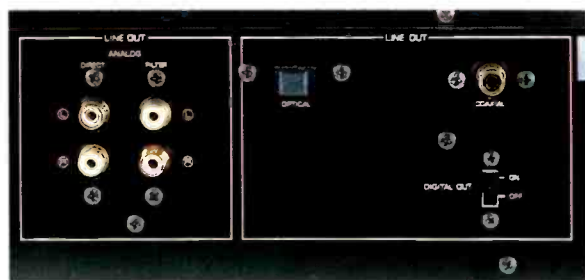
Yamaha's CDX-1110U CD player has both coaxial and optical digital outputs that are selected by a rear-panel switch.
