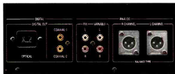
Denon's DCD-3300 CD player offers one optical and two coaxial digital outputs.
