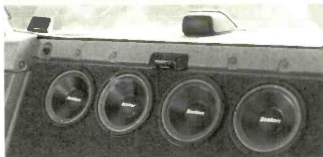
Boston 761 two-way component systems are installed in the rear: the 6 1/2" woofers in the deck (not visible) and the Varimount tweeters in their wedge-shaped housings on the deck, facing forward. (Also shown here, the four Boston 780LF subwoofers.)
