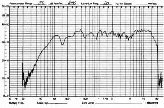
Figure 8. Frequency response of the KEF C10 speaker, measured on-axis.
