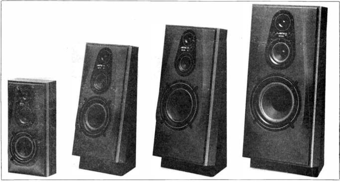
The resulting baffle construction comprises two layers of vacuum-formed polystryrene with the concrete-like material injection moulded between to form a sandwich 25 mm thick. The outer polystyrene skin of the baffle incorporates a moulded anti-diffraction pattern to preserve the stereo image at the upper end of the audio range. See Figure 2.
