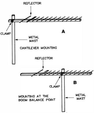
Figure 9. Horizontal polarisation mounting arrangements — (a) shows cantilever mounting, while (b) shows mounting at the boom balance point. In both instances, a metal mast may be used.
