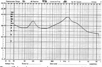
Figure 12. Impedance versus frequency response of the C10 speaker.
