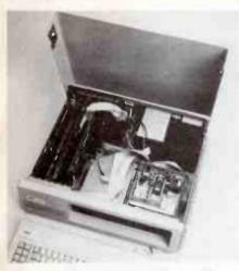
Showing the rear-hinged flip-up lid and the general internal arrangement.
