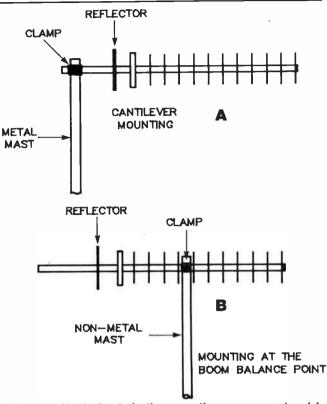
Figure 8. Vertical polarisation mounting arrangement — (a) shows cantilever mounting where a metal mast is employed, (b) shows mounting at the boom balance point, but here a non-metallic mast must be used.
