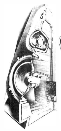
Figure 4. Showing the asymmetric cabinet design of the new Jamo Digital Monitor CBR series speakers. No sides are parallel so as to reduce cabinet internal resonances. The front panel is angled to align the acoustic centres of the drivers to obtain 'time coherent' sound radiation. The photograph shows a cutaway view of the CBR 200.
