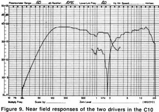
Figure 9. Near field responses of the two drivers in the C10 speaker.
