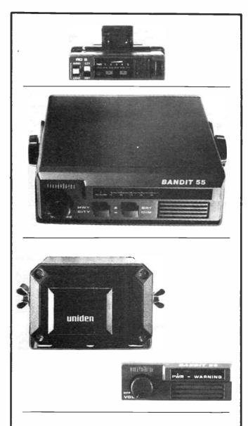
Typical of the radar detectors on the market are these three units, manufactured in Asia by the Uniden Corporation of America. All operate off the 12 Vdc car supply. These units were supplied by Dick Smith Electronics.
