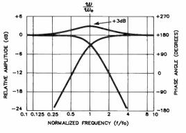
Figure 2, the second-order crossover results. A quick glance at the transfer functions and resulting overall frequency response shows that this crossover is entirely unsuitable for use in loudspeakers. The overall frequency response shows an infinitely deep hole at the crossover point which is caused by phase cancellation between the outputs of the filter sections.
