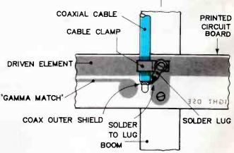
Figure 7. How the feedline connection is terminated and the driven element assembled.
