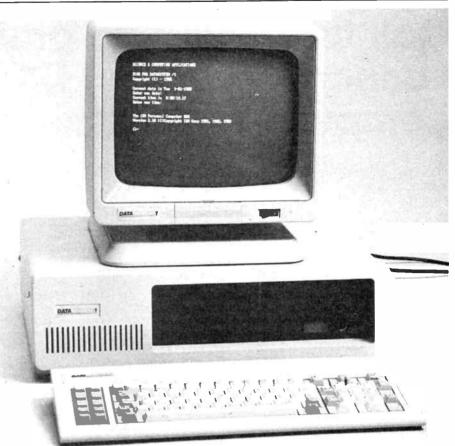
The DataSystem/1 PC compatible looks much as you'd expect. It features a flip-up lid hinged at the rear for convenient access to the eight-slot motherboard.
