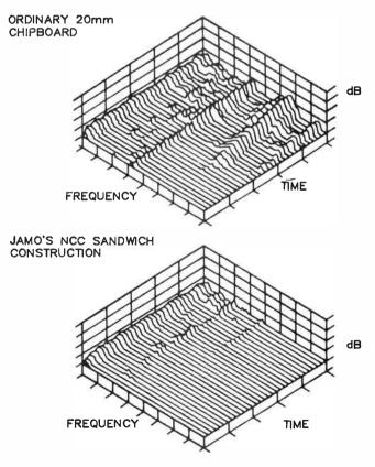
Figure 3. Comparison of the time decay spectral response to a pulse applied to 20 mm chipboard (upper graph) and Jamo's NCC sandwich connstruction (lower graph). Both materials were 'hit' with a pulse containing all frequencies between 20 Hz and 7 kHz. These vibration measurements show the damping characteristics of the two materials. The less 'landscape' there is, the fewer resonances there are, and hence the better the damping.
