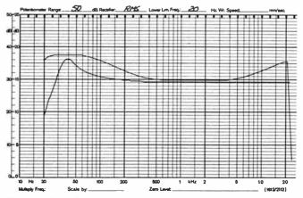
Figure 6. Superimposed curves of the loudness (upper trace) and bass eq (lower trace) switches of the NAD 1155.
