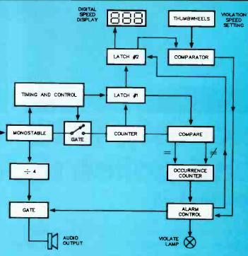
displays it, etc. There is provision for sounding an alarm if a preset value is exceeded and to latch the number in the counter if desired when this condition occurs.
