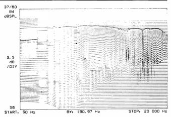
Figure 16. Impulse response of the C10 speaker shows only minor irregularities around 4 kHz and 7.35 kHz.
