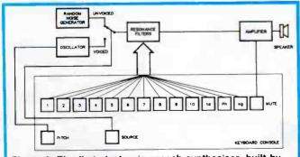
Figure 2. The first electronic speech synthesiser, built by Homer Dudley's team at Bell Labs in the US in 1939. Dubbed the ''Voder'', it was 'played' by keys and a pitch pedal, producing quite good results when used by a skilled operator. This was the forerunner to the modern-day ''Vocoder'' occasionally used in music recording. microprocessor that speech synthesis came out of the laboratories.
