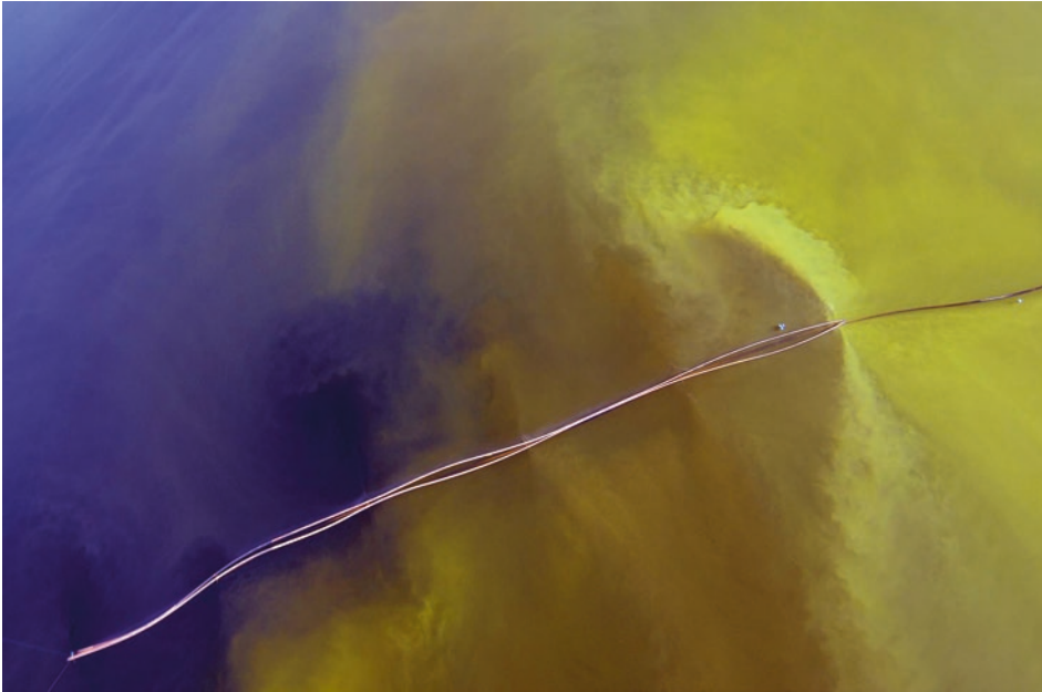
Fig. 6.4 Injection of slaked lime into Lake Scheibe, Germany, in November 2010 via hose lines and a land-based injection station. (Image width about 500 m; Photo: Peter Radke, LMBV)
