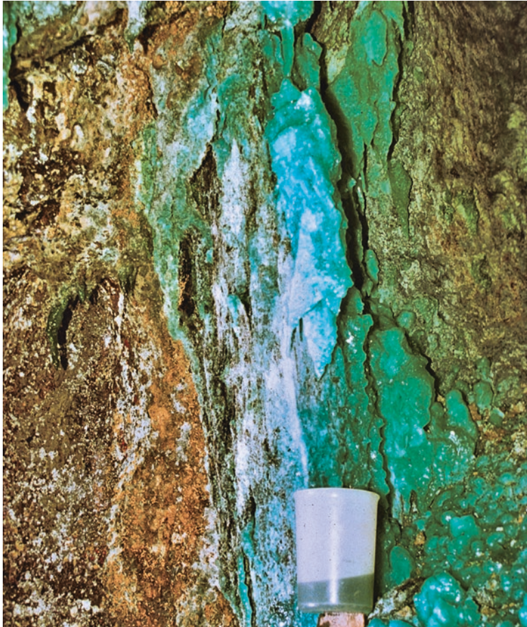
Fig. 1.5 Stalactite of melanterite above the puddle where Alpers and Nordstrom measured the mine water to have a pH of -3.6 . The mine water in the 2-L-beaker has a pH of -0.7 and a temperature of 35\text{ }^{\circ}\text{C} . (Pers. comm. Kirk Nordstrom 2019; photo: Kirk Nordstrom & Charly Alpers). Scale: Plastic beaker
