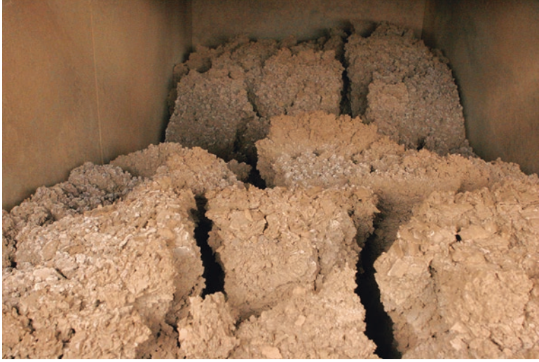
Fig. 3.8 Sludge dewatered by filter presses. (Acid rock drainage treatment plant Halifax Airport, Nova Scotia, Canada; image width approx. 1 m)
