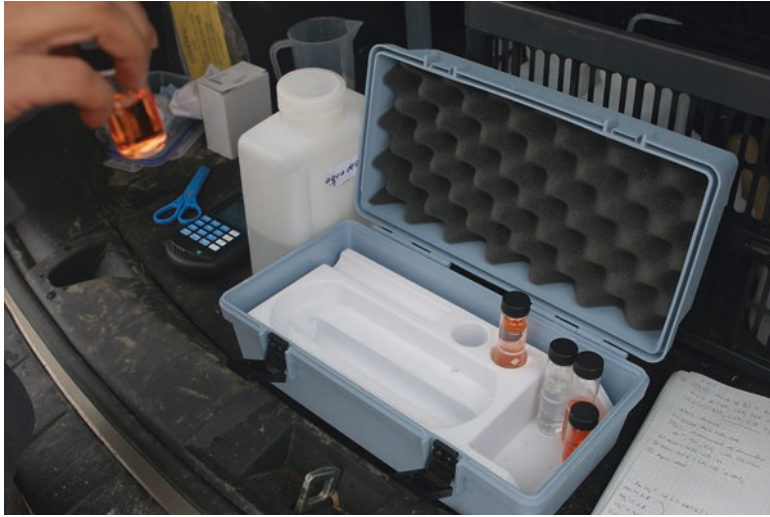
Fig. 2.14 Photometric on-site analysis of total iron and \text{Fe}^{2+}
