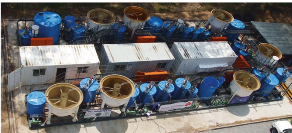
Fig. 3.25 SAVMIN™ pilot plant at Western Utilities Corporation’s Mogale gold mine in South Africa. (From Roger Paul: “Presentation to the Parliamentary Committee on Water and Environmental Affairs” – 7/8 September 2011)
