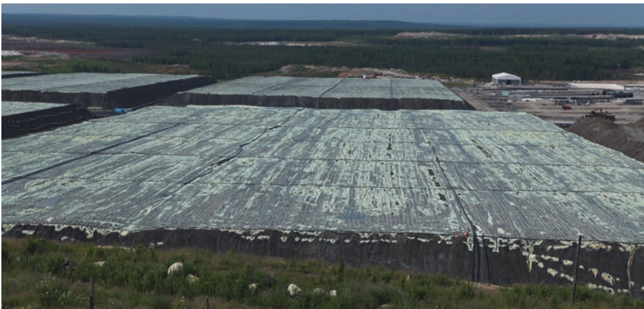
Fig. 5.5 Heap leaching at the Finnish Terrafame nickel mine (formerly Talvivaara)
