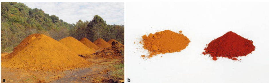
Fig. 7.6 Waste rock piles with ochre from a passive mine water treatment after dewatering and drying (a) and dried as well as burnt ochre (b) (Photos: Bob Hedin)
