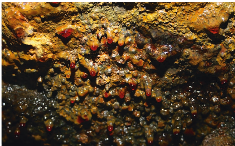
Fig. 1.7 Drops of acid mine drainage with pH 2 at a gallery roof in the former Glasebach mine in Straßberg/Harz, Germany. Second level: area of the pyrite passage. (Image width approx. 20 cm)
