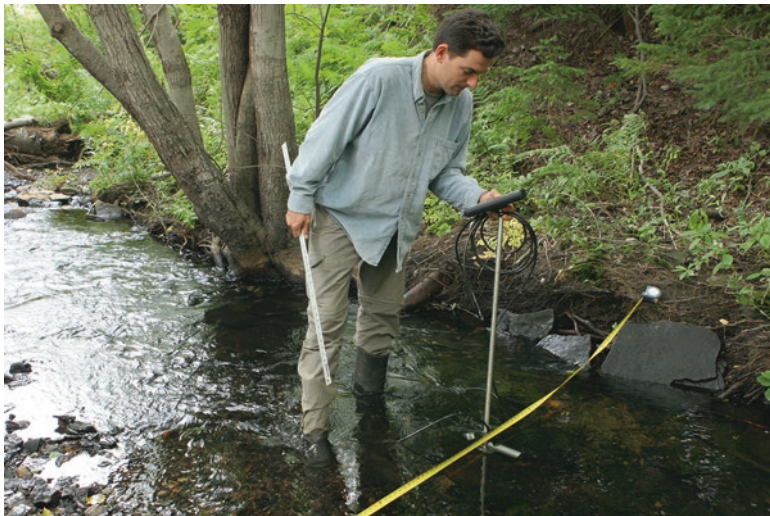
Fig. 2.9 Flow measurement with an acoustic digital flow meter in a mine water influenced stream (Cape Breton Island, Nova Scotia, Canada). The operator correctly stands downstream of the meter and holds the meter far away from the body to avoid interfering with the flow as far as possible
