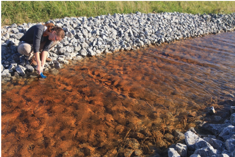
Fig. 4.6 Open limestone channel with iron hydroxide precipitates at the mine water discharge of the former Dominion No. 11 coal mine on Cape Breton Island, Nova Scotia, Canada
