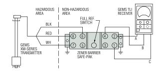
P/N 54805 in a continuous liquid level monitoring system.
