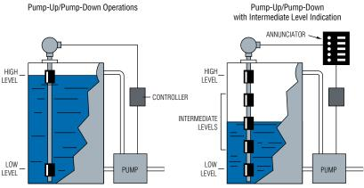
Using GEMS Custom Length level switches, junction boxes, solid-state relays and annunciators, complete liquid level control systems are easily configured.
