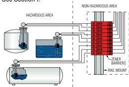
Any non-voltage-producing sensor or switch is rendered intrinsically safe for hazardous locations when properly connected to the output of GEMS Zener Barriers. These are described in Section I.
