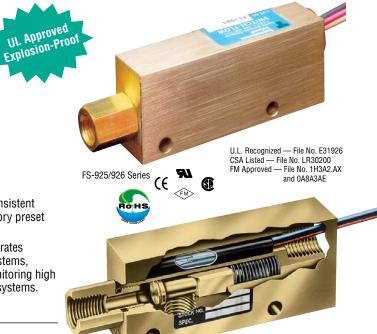
Both the FS-925 and FS-926 use a spring-loaded piston to detect positive flow with great precision. They act upon direct fluid flow and will not show "false-positive" flow indication as can happen with sensors using indirect sensing methods such as pressure measurement. The FS-926 incorporates an additional lap-fitted piston for very low flows; see below.
