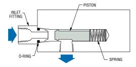
Accumulation of foreign debris should periodically be removed from these switches. GEMS' designs provide for easy piston and spring removal for this occasional cleaning. Recommended cleaning procedures are provided in the Instruction Bulletin shipped with each unit. 150 micron filtration is recommended for the FS-150 Series; 100 micron for FS-380, 50 micron filtration is recommended for all other piston type switches.
