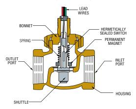
As liquid flow increases to the actuation setting, a magnet-equipped shuttle is displaced. When displaced by fluid flow, this shuttle actuates a hermetically sealed, SPDT or SPST reed switch within the unit stem. A compression spring or gravity provides shuttle return when flow decreases.
