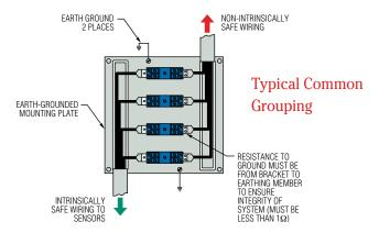
The only maintenance normally required is routine inspection approximately every two years or less to check integrity of earth-grounding and electrical connections, and to make sure the unit is clean.
