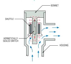
The FS-400P Series is an inexpensive alternative for plastic piping systems. Units are available in clear PVC housings. The clear version, with a bright red shuttle, provides highly visible affirmation of flow status. Low-cost, all PVC versions are for use in systems where liquid pressures are below 120 PSIG and temperatures do not exceed 120°F. An easily removed, one-piece bonnet and shuttle assembly for quick clean-out is featured.
