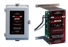
These units feature a large 4-digit display and bright LED bargraph to visually clarify relative tank content level.
