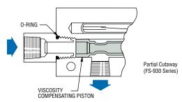
When temperatures of viscous fluids change, so do their flow properties. With viscosity lowered by increasing temperature, a greater flow is generally required to create actuation pressure differential. A unique patented piston within GEMS FS-930 Series switches accommodates these changes in fluid viscosity while maintaining accurate switch actuation. Units can detect flow rates with 20% accuracy for liquid viscosities between 40 to 1000 SSU.
