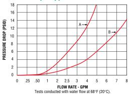
Flow Range A .13 - 2.6 GPM .5 - 10 LPM Flow Range B .26 - 9.2 GPM 1 - 35 LPM
