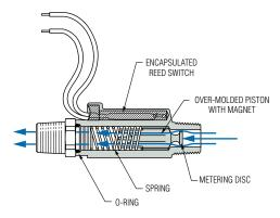
The key to the excellent flow qualities of the FS-150 and FS-380 Series switches is the dual diameter internal bore. At flow rates below the actuation point, the fluid passes around the piston and metering disc within the "metering bore." As fluid flow increases past the actuation point, the metering disc enters the "flow bypass bore" where the increased diameter provides generous flow paths. The result is a low pressure drop for high flow rates and less susceptibility to fouling.
