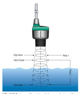
UCL-510 Series multi-point switches are designed for easy automatic tank "Hi/Lo" liquid level control. They combine non-contact continuous sensing with four SPST relays; actuation points are field adjustable in a range to 49 inches.
