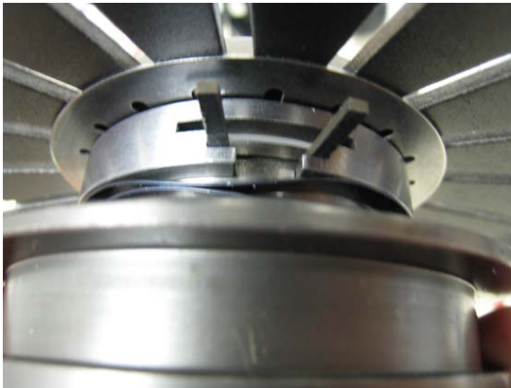
Retaining Clip shown “latched” into the closed position.
