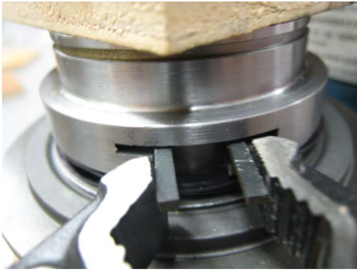
Retaining Clip in compressed position so tabs can pass through gate. (Diaphragm removed for clarity of photo)
