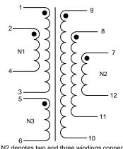
N1, N2 denotes two and three windings connected in parallel. Terminals 1+2, 3+4, 7+8+9 and 10+11+12 must be tied as solder bridging is allowed.
