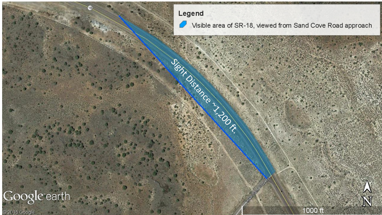
Figure 3 – Sand Cove Road Sight Distance, Looking North
