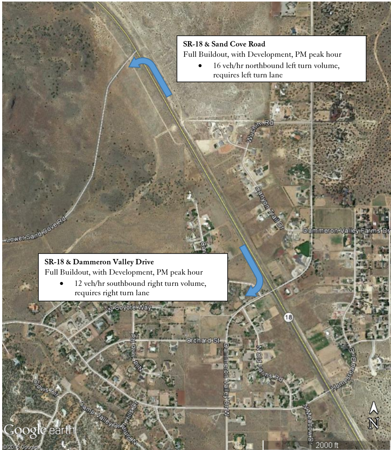
Figure 4 –Turn Lanes Required
