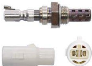
250-22002 DODGE (4) 1989-91 / EAGLE (4) 1989-94 HYUN (4) 1989-93 / MITSU (4) 1989-94 PLY (4) 1989-94 Unheated Sensor, 650mm 2wire
