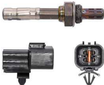
250-24383 HYUN (4,6) 1997-03 / KIA (6) 2002-05 Heated Sensor, 820mm 4wire
