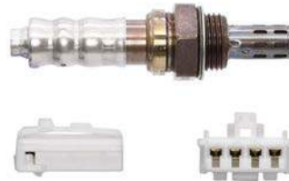
250-24083 CHRY (4) 1995-99 / DODGE (4) 1995-99 EAGLE (4) 1995-98 / MITSU (4) 1995-99 Heated Sensor, 630mm 4wire
