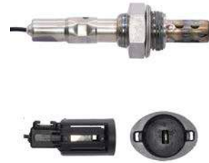
250-21004 AMC (4,6) 1981-87 / FORD (4,6,8) 1984-86 JEEP (4,6) 1981-86 / MER (4) 1984-86 MERKUR (4) 1985-89 / REN (4) 1983-87 Unheated Sensor, 400mm 1wire
