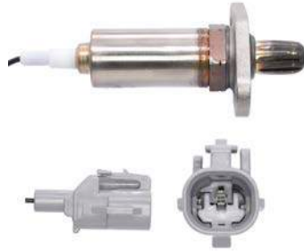
250-21054 LEXUS (6) 1992-94 / TOY (4,6) 1992-95 Unheated Sensor, 450mm 1wire
