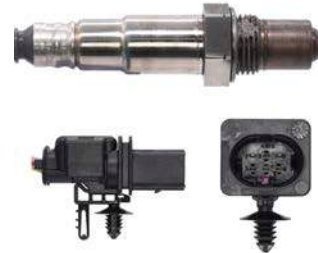
250-25051 AUDI (12) 2008-09 / PORSCHE (6) 2011-18 VW (6) 2011-15 Wideband Sensor, 1575mm 5wire
