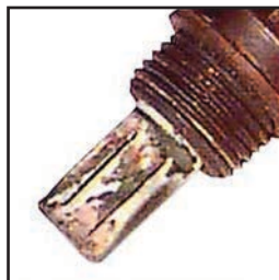
Ethylene Glycol (Antifreeze) Contamination
