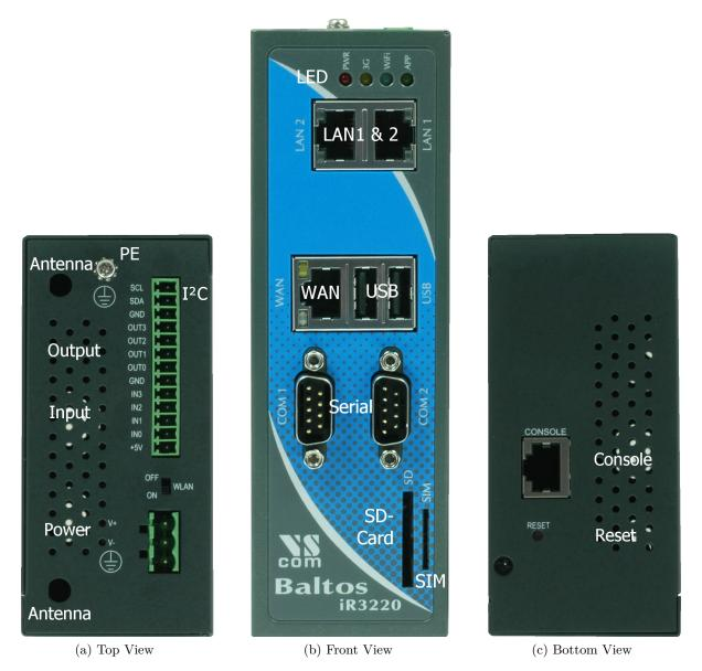
Figure 2: Appearance VPNRouter iR 3220
