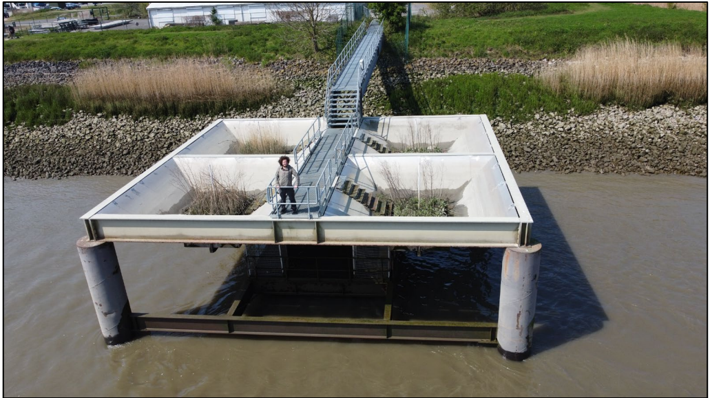
Figure 5.3: Picture of the mesocosm set-up at low tide taken 3.5 years after the start of the experiment showing the four units containing the soil monoliths with different treatments. From left to right and top to bottom: CTRL: control treatment, no tillage and no amendments, REED: tillage and amendment with reed cuttings, WOOD: tillage and amendment with wood chips and PLOW: tillage and no amendments. Photo taken by Tim van den Broeck.
