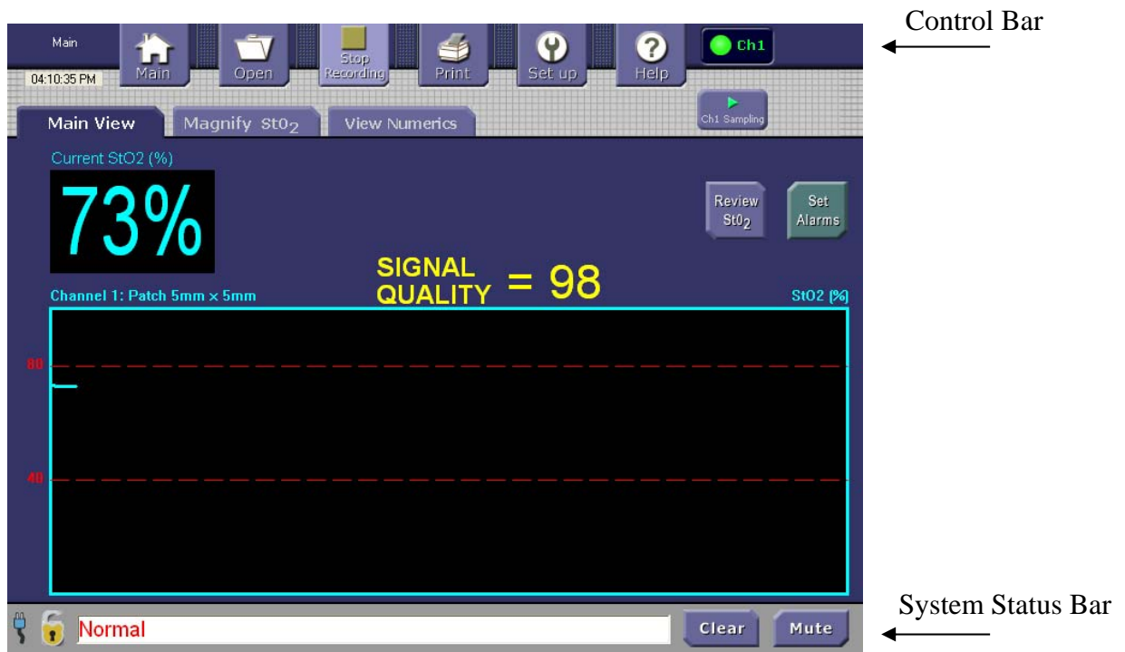
Figure 4. Main Screen, with Control Bar at Top and System Status Bar at Bottom
