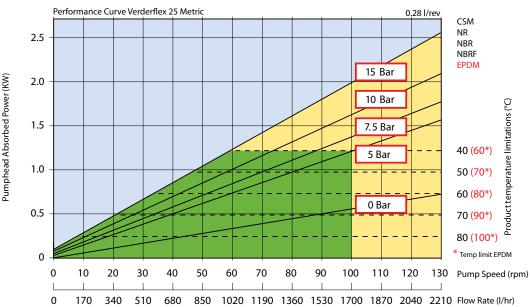
Displacement 0.28 l/revolution, Capacity is speed x 17 in l/hr. Minimum starting torque required: 115 Nm
