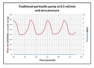
A standard peristaltic pump gives quite significant flow rate fluctuations. This is especially important with two pumped reagents – if these flow fluctuations were out of phase there would be huge swings in reaction stoichiometry entering the reactor.
