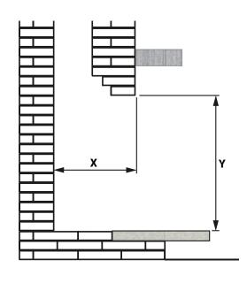
Check that masonry step does not interfere with install dimensions or vent pipe.
