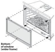
4. If the Hot Glass Warning plate has been removed from the front lower corner of the window, reinstall it by sliding it between the glass and the frame as indicated.
