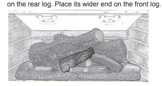
7. Identify the left cross log; it has a hole under its narrow end. Place its narrow end on the pin located
