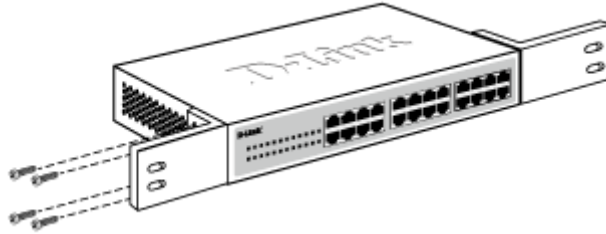
Figure 3-2 – Attach the mounting brackets to the switch
