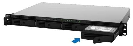
Note: Make sure the drive tray is completely inserted. Otherwise, the drive might not function properly.
