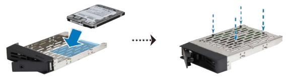
3 Insert the loaded hard drive tray into the empty hard drive bay.
