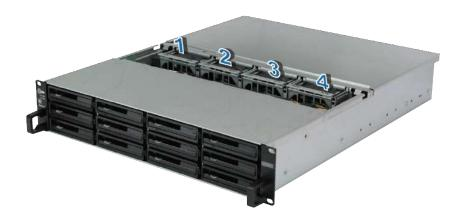
4 Find the malfunctioning fan and lift it upward to remove.
