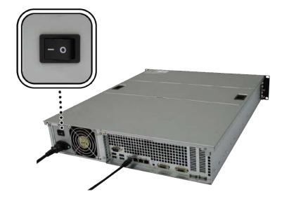
4 Press the power button to turn on the RackStation.
