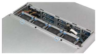
**b** Remove the two screws located on the back. Then slide the top cover in the direction indicated below and lift.
