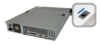
3 Lift and remove the fan cover.
