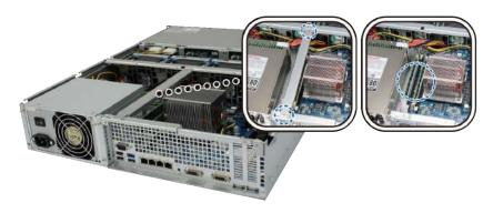
*Important:* Removing the cover will expose sensitive internal components to possible harm. Please avoid touching any other components when adding or removing memory.
