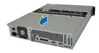
**c** Remove the screws of the securing bracket and remove the securing bracket to reveal the RAM slots.
