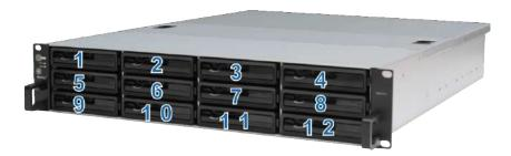
**Note:** If you want to create a RAID volume, we recommend all installed drives be the same size in order to optimize drive capacity usage.
