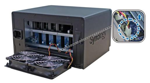
$\boldsymbol{c}\,$  Remove the 4 screws that secure the malfunctioning fan, and then remove the fan.
