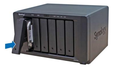
Note: Make sure the tray is pushed in all the way. Otherwise, the drive might not be able to function properly.
