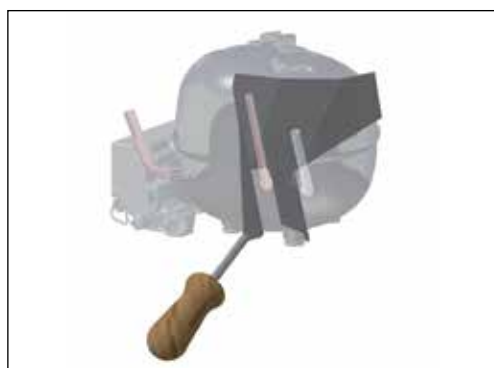
Use brazing protection shield
