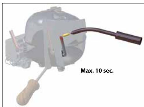
Use brazing protection shield
