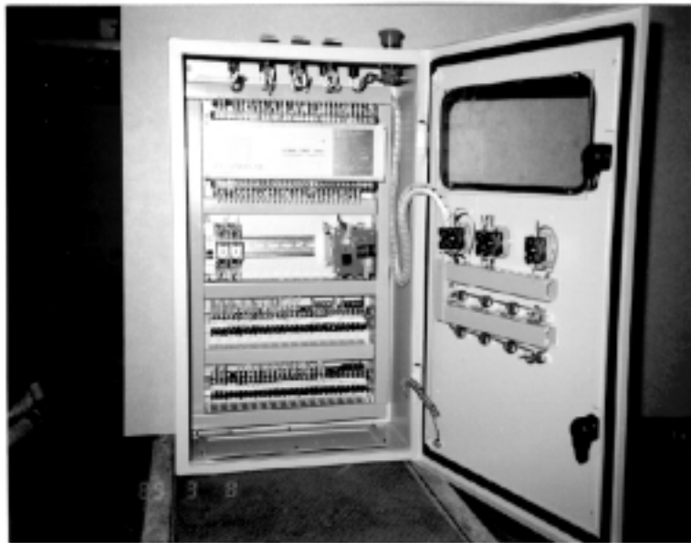
Fig. 1.5: Typical PLC Control Panel
