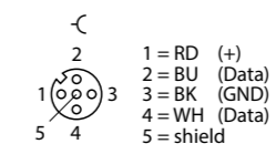
RFID channels (X0...X3) - Connectors .../S2503
