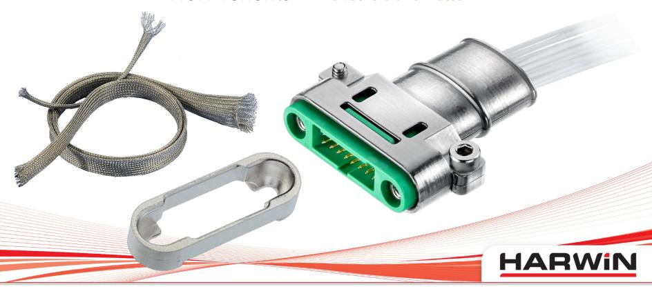
The strong and lightweight machined aluminium backshells provide additional strain relief. They are designed to accommodate flexible, abrasion resistant, metal braiding and are supplied with tie-bands to attach such braiding to the shell. The backshells, together with the braiding, provide shielding for enhanced electrical continuity and effective EMI/RFI protection.
