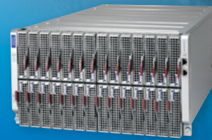
6U MicroBlade™ Up to 112x 1S or 28x 2S Nodes
