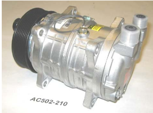
AC502-210 Compressor, TM-16, (8) Grv., Poly-V, 12 VDC, Ear Mount, Vertical O-Ring, Monolithic Head, (Superseded to 18-00093-05)
