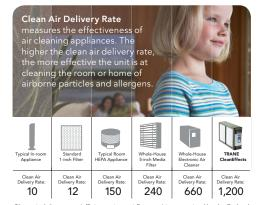
Clean air delivery rate (efficiency times airflow rate) is recognized by the Federal Trade Commission (FTC) and the Environmental Protection Agency (EPA) as a fair and objective measure of various air cleaner technologies. Ratings reflect cubic feet per minute of clean air delivered for a typical 3-ton heating and cooling system: the higher the value, the more effective the air cleaner.
